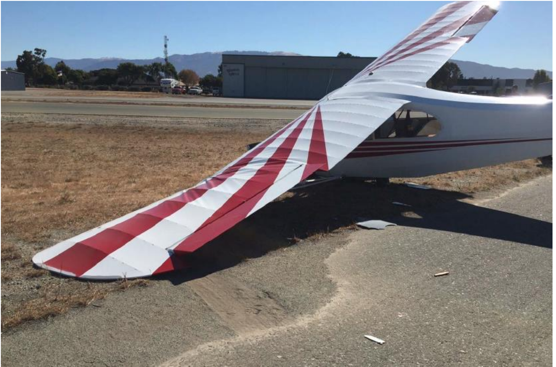
Photo 1 – View of damaged left wing (Photo courtesy of the FAA)
