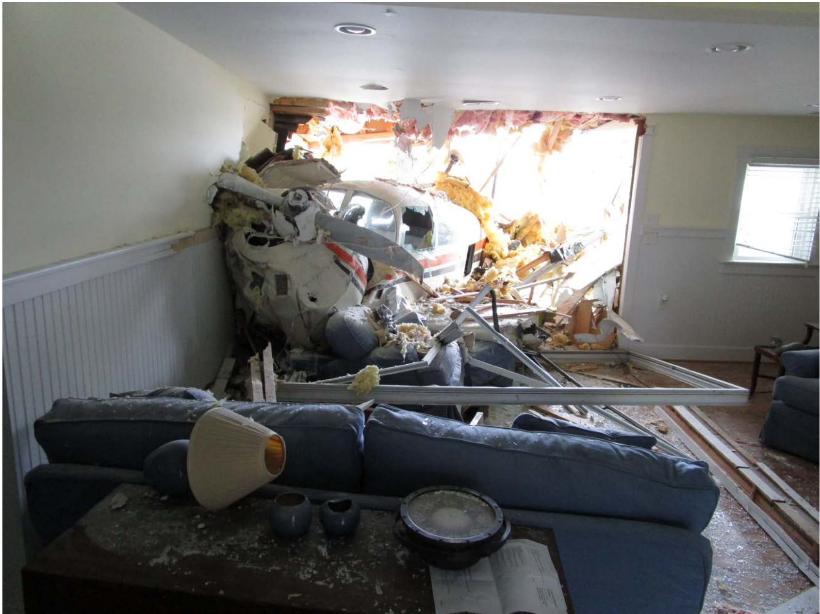
Photo 1 – View of damage to left wing (Courtesy of FAA)
