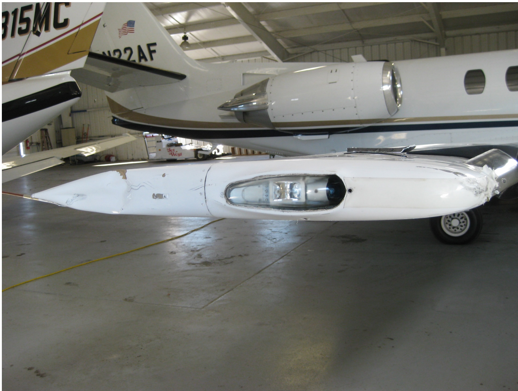
Photo 2 – Image of right wing tip damage to airplane (Courtesy of FAA)
