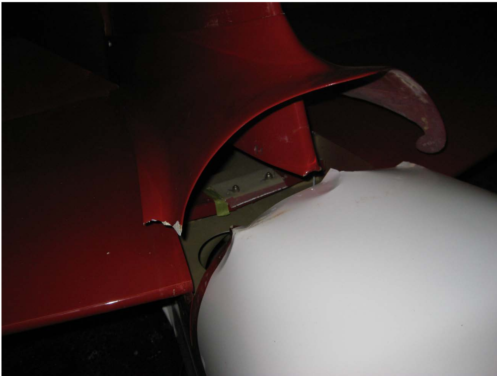
Photo 1 – View of damage to aft bulkhead and vertical stabilizer (Courtesy of FAA)
