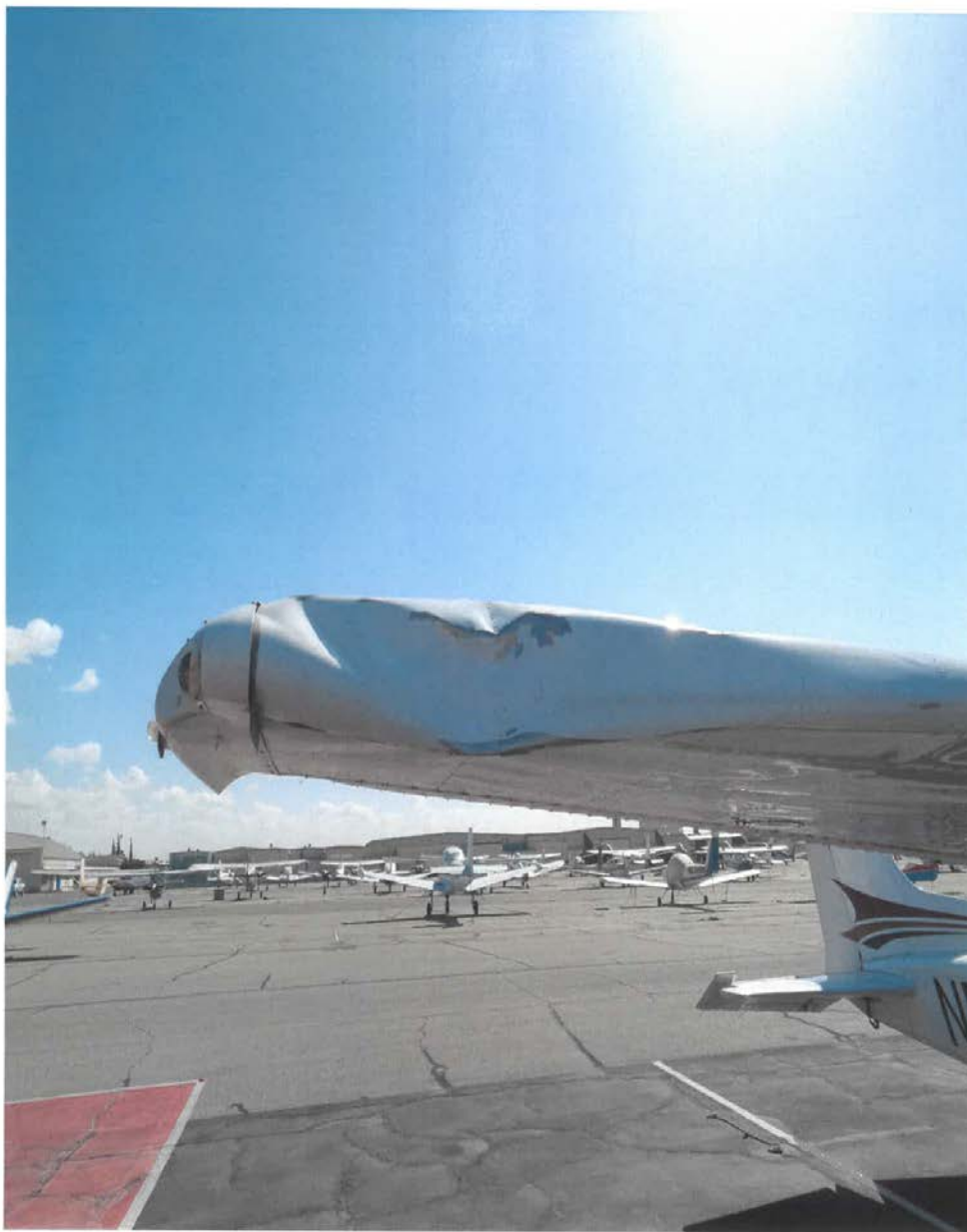
Photo 1 – View of damaged right wing leading edge (photo courtesy of airport maintenance)
