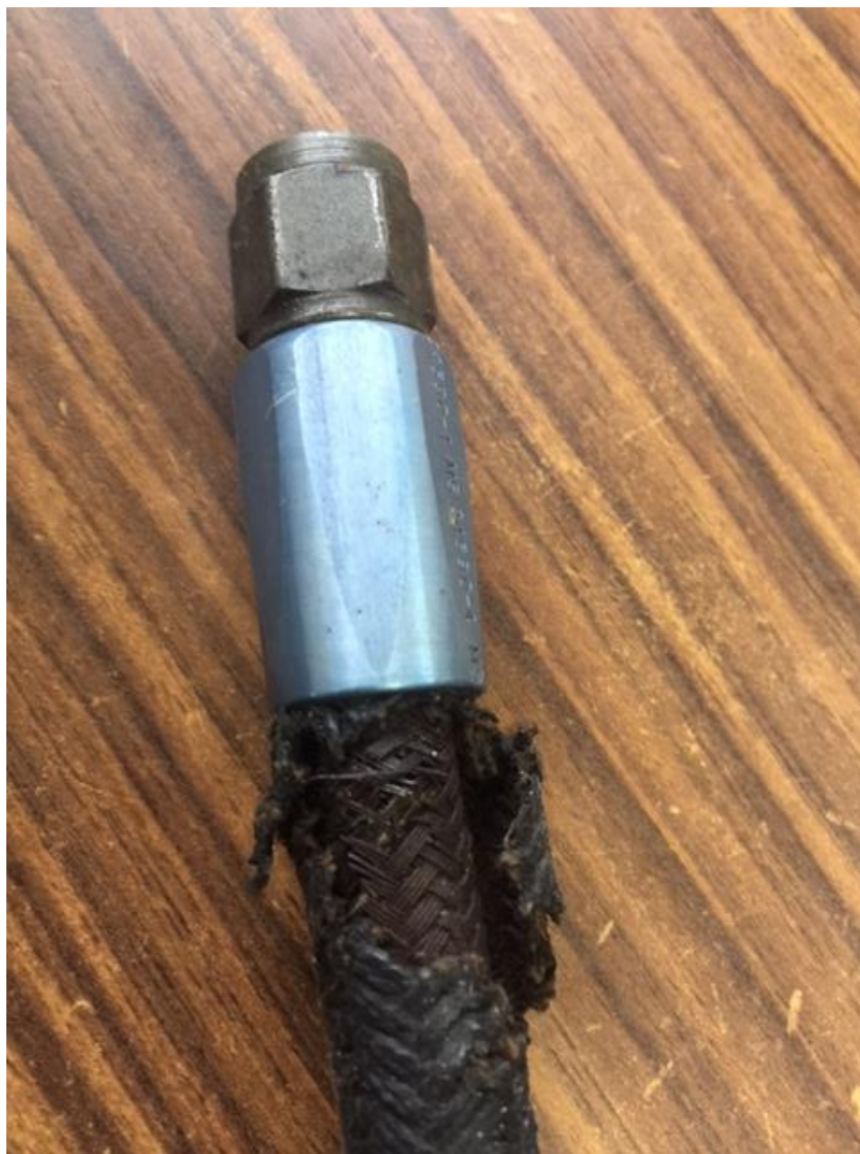
Photo 2 - View of right inboard main landing gear door actuator hose (photo courtesy of the Operator)
