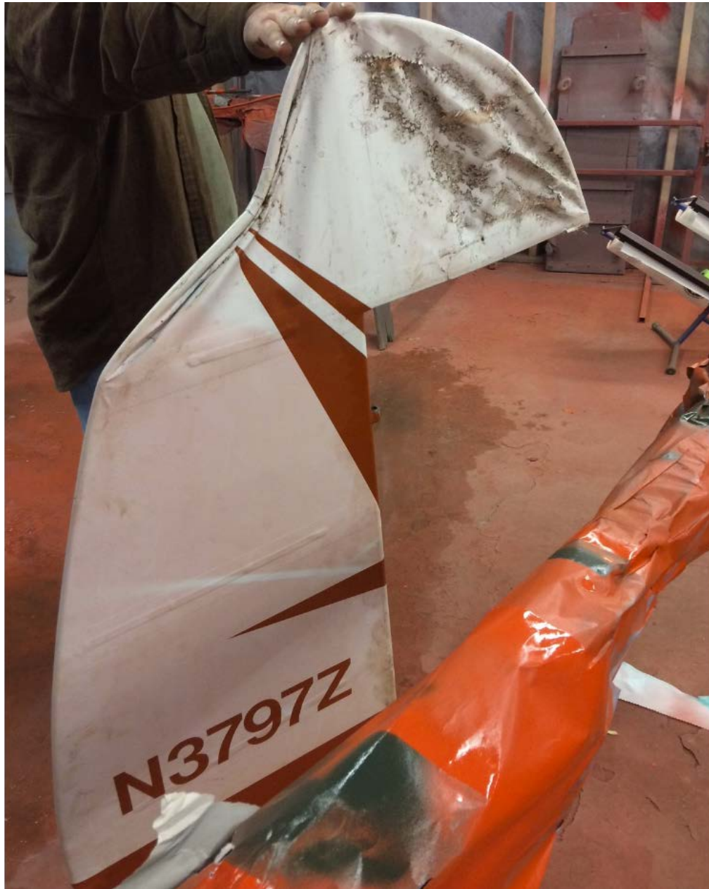
Photo 1 – View of replaced rudder (Courtesy of FAA)
