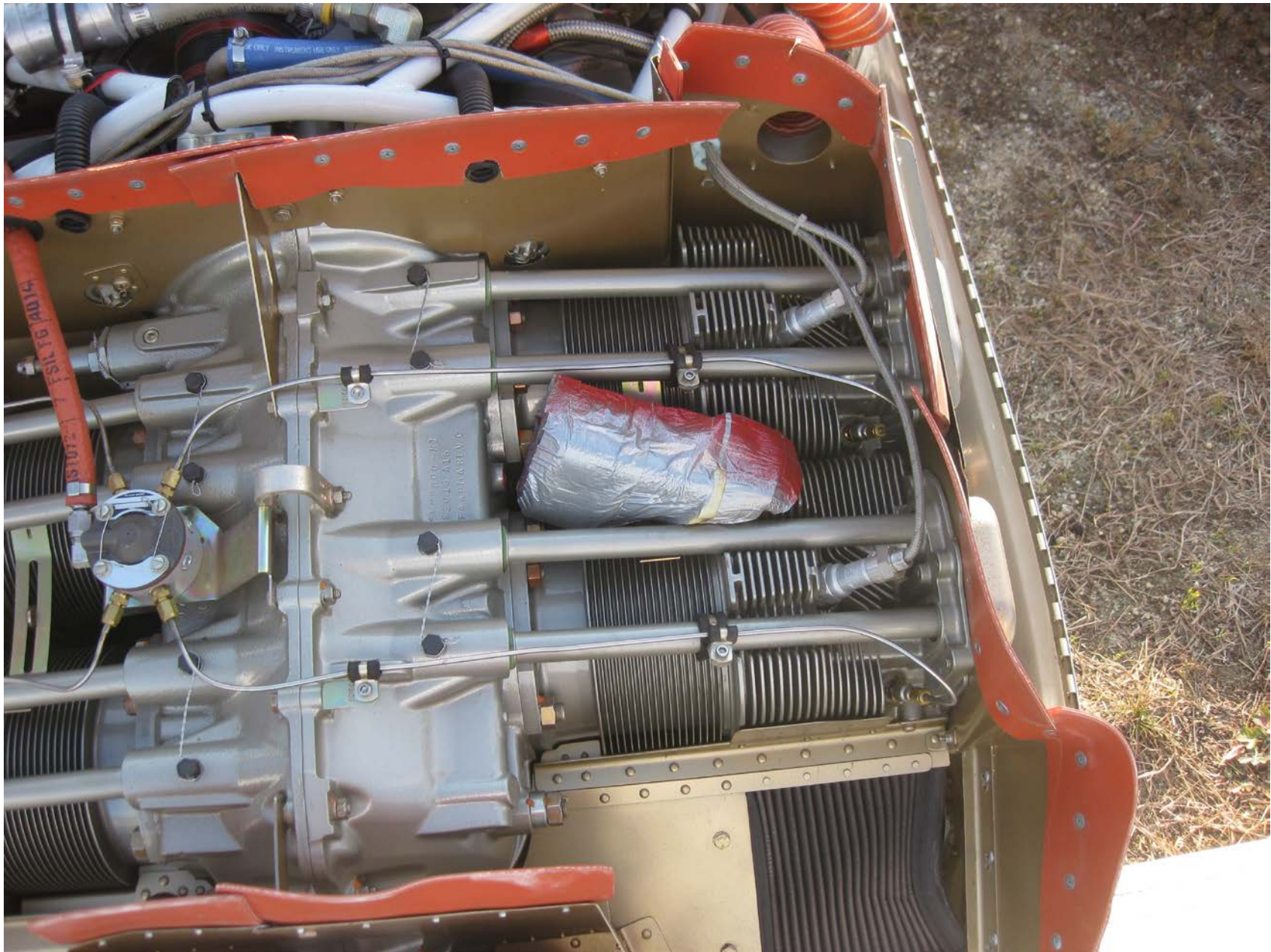
Photo 3 – Engine Cowl Plug as Found After Accident (Photo Courtesy of FAA)
