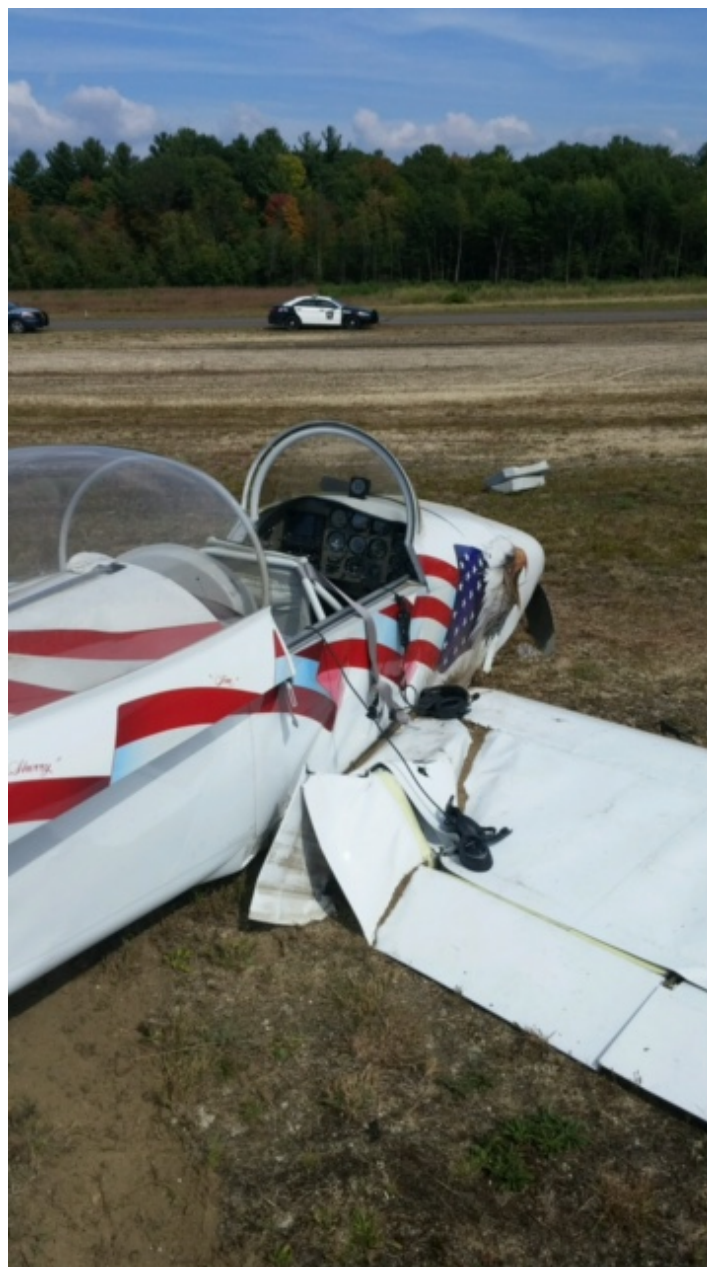
Photo 2 - Substantially Damaged Right Wing (Photo Courtesy of FAA)
