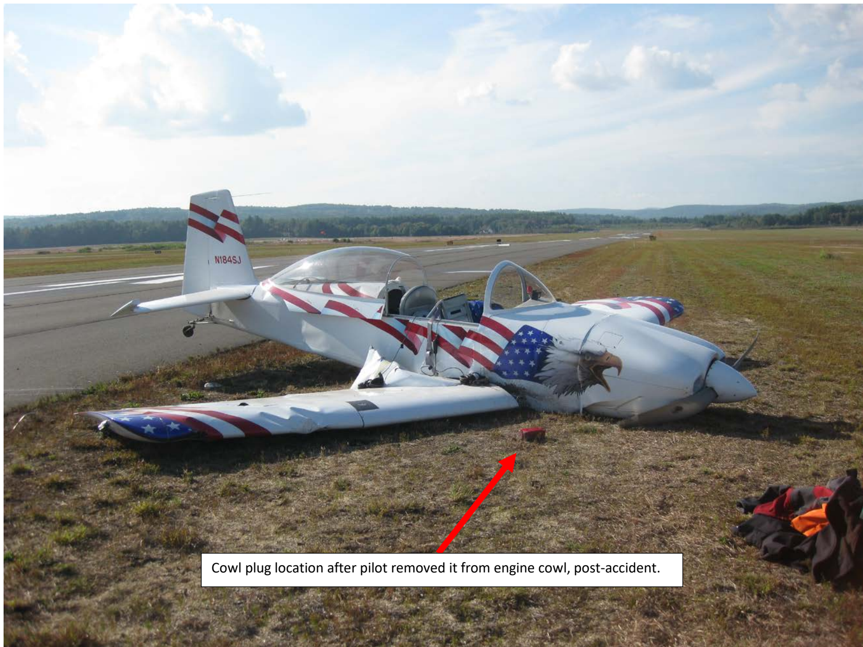
Photo 4 – Overview of Accident Airplane and Cowl Plug (Photo Courtesy of FAA)
