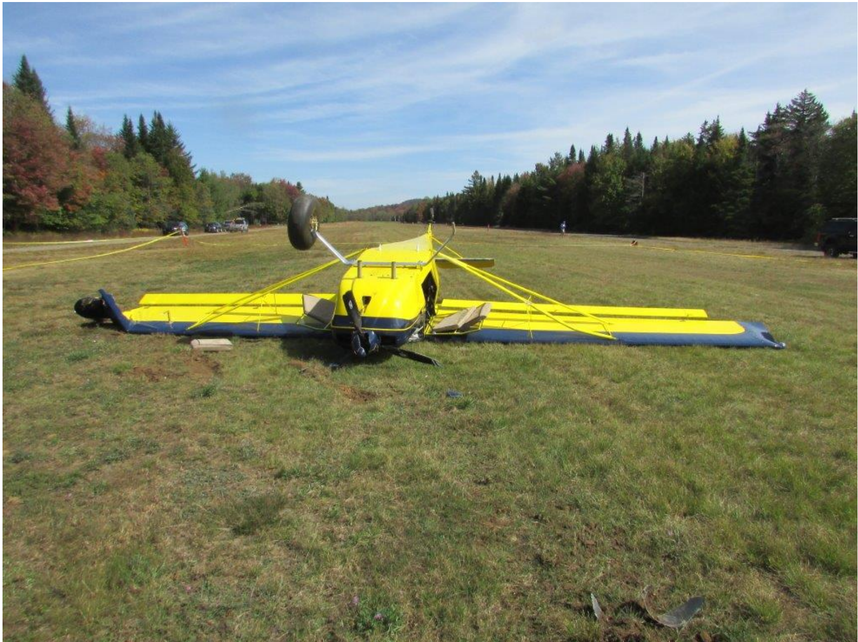
Photo 1 – View of damage to the left wing and right-wing strut (Courtesy of FAA)
