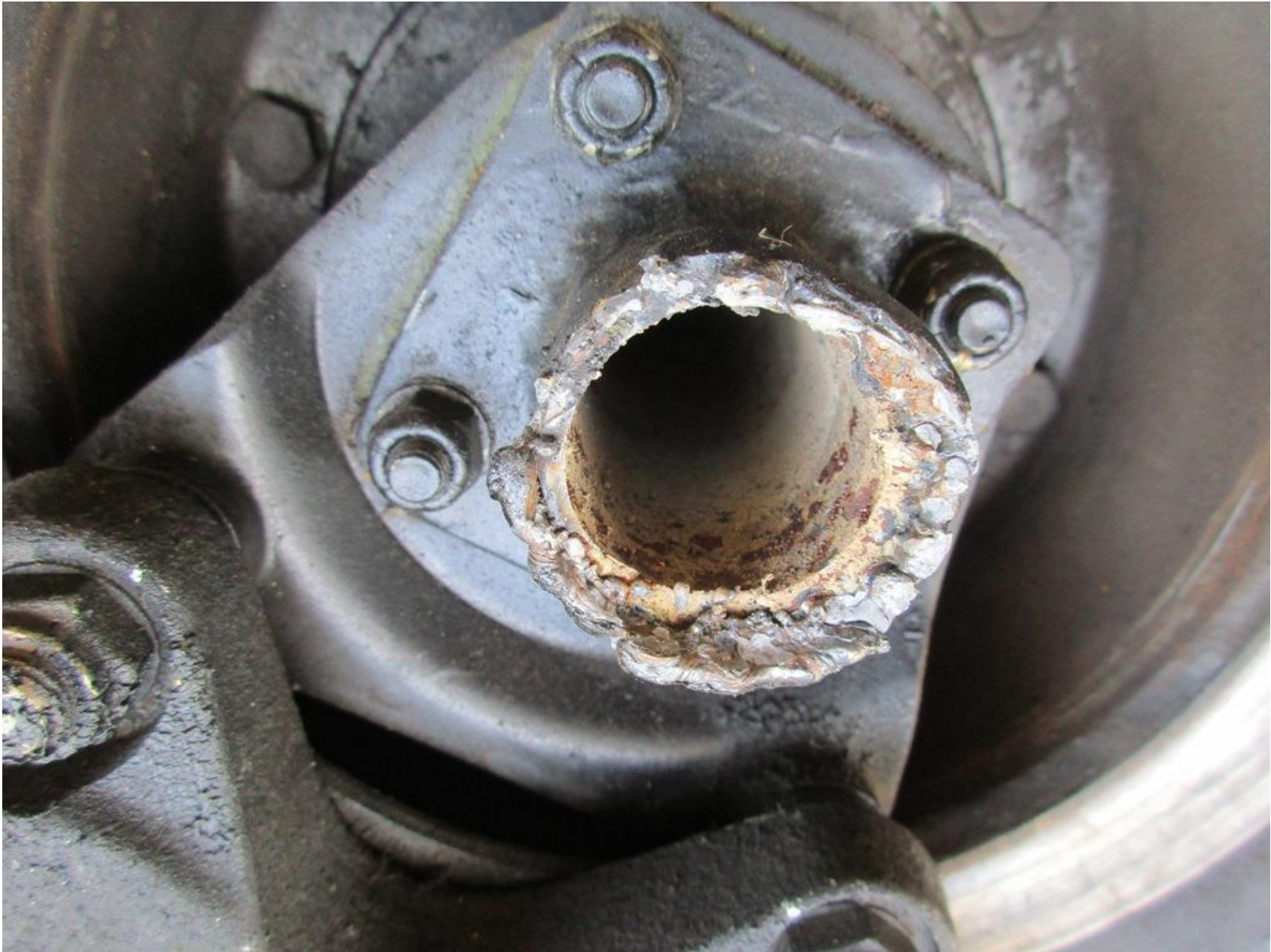
Photo 2 - View of broken weld on left main landing gear axle (photo courtesy of the pilot)
