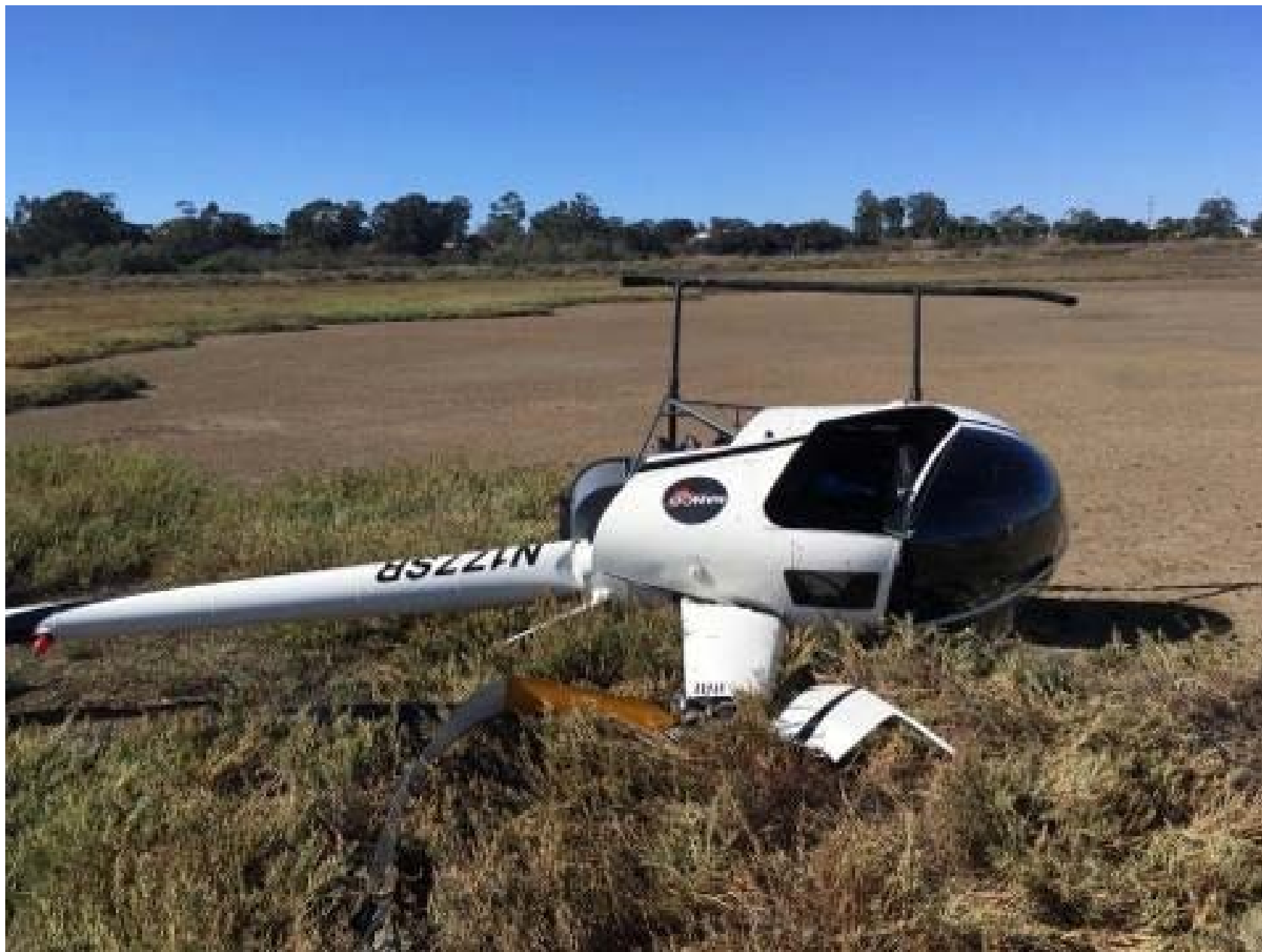
Photo 1 – View of damage to the tailboom (Courtesy of FAA)
