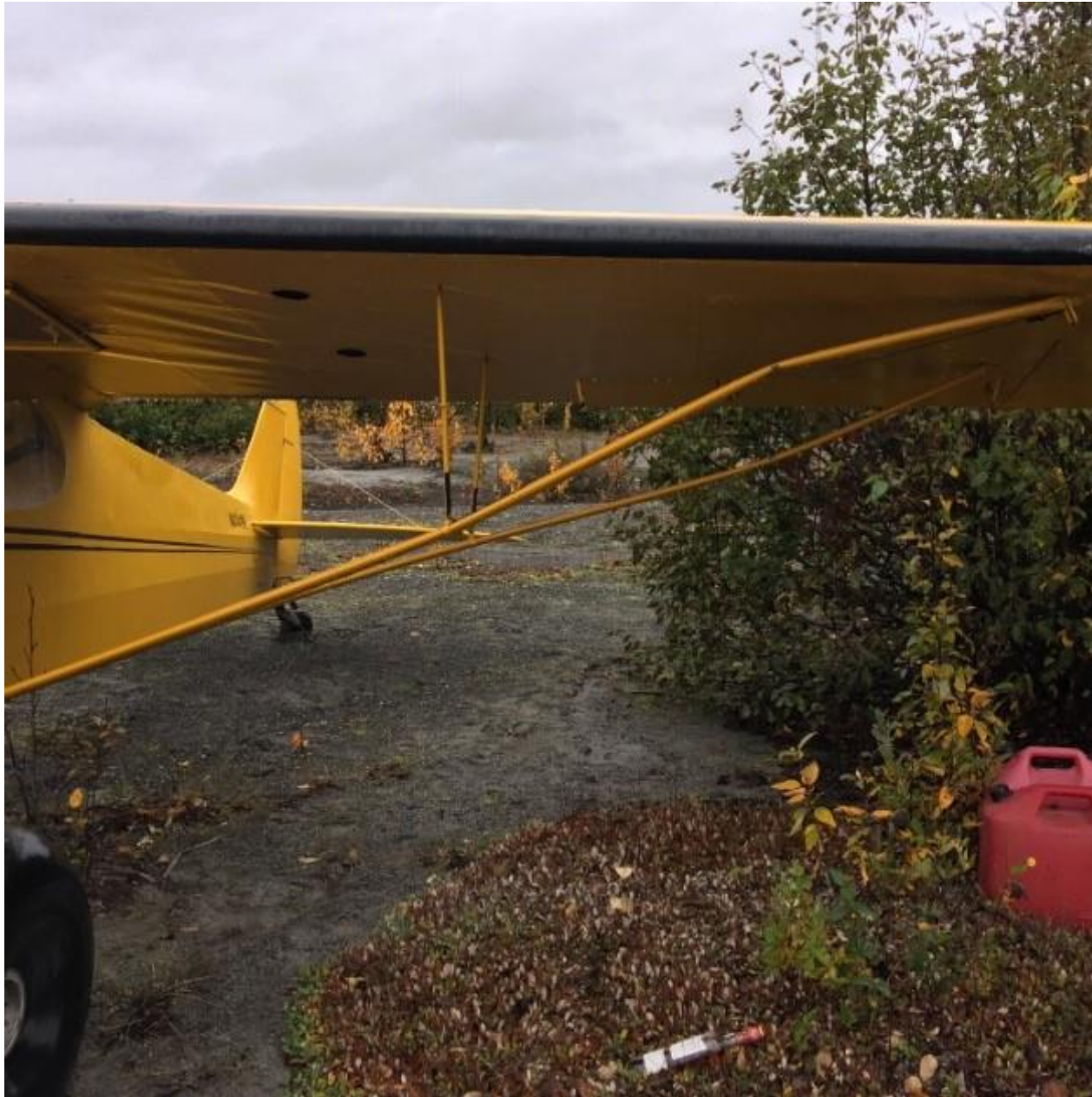
Photo 1 – View of damaged left wing lift strut (Photo courtesy of the pilot)
