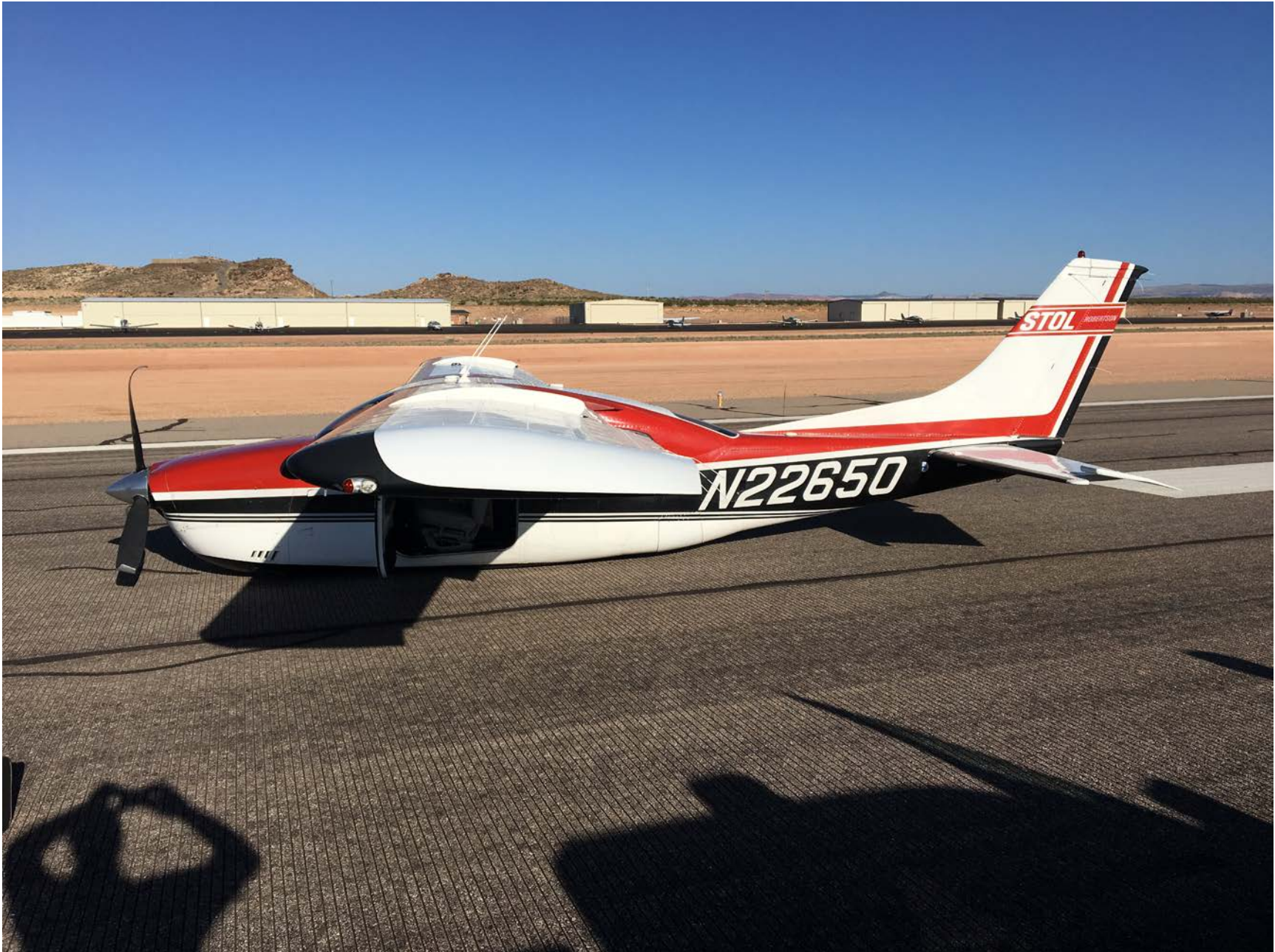
Photo 1 – View of airplane after gear up landing (photo courtesy unknown)
