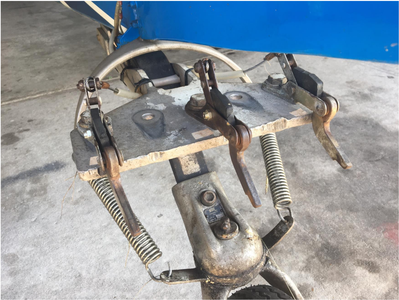
Photo 2 - View of the three-hook banner release mechanism (photo courtesy of the Operator)
