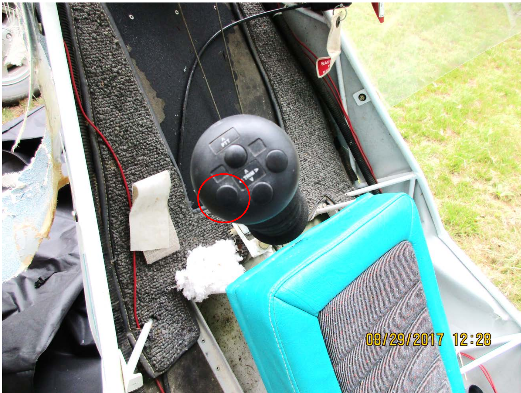
Photo 4 – Left Trim Button Located of Control Stick (Photo Courtesy of FAA)
