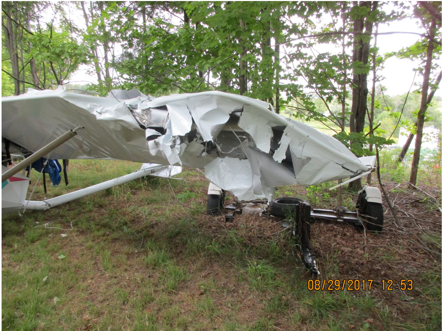
Photo 2 - Damaged Left Wing (Photo Courtesy of FAA)
