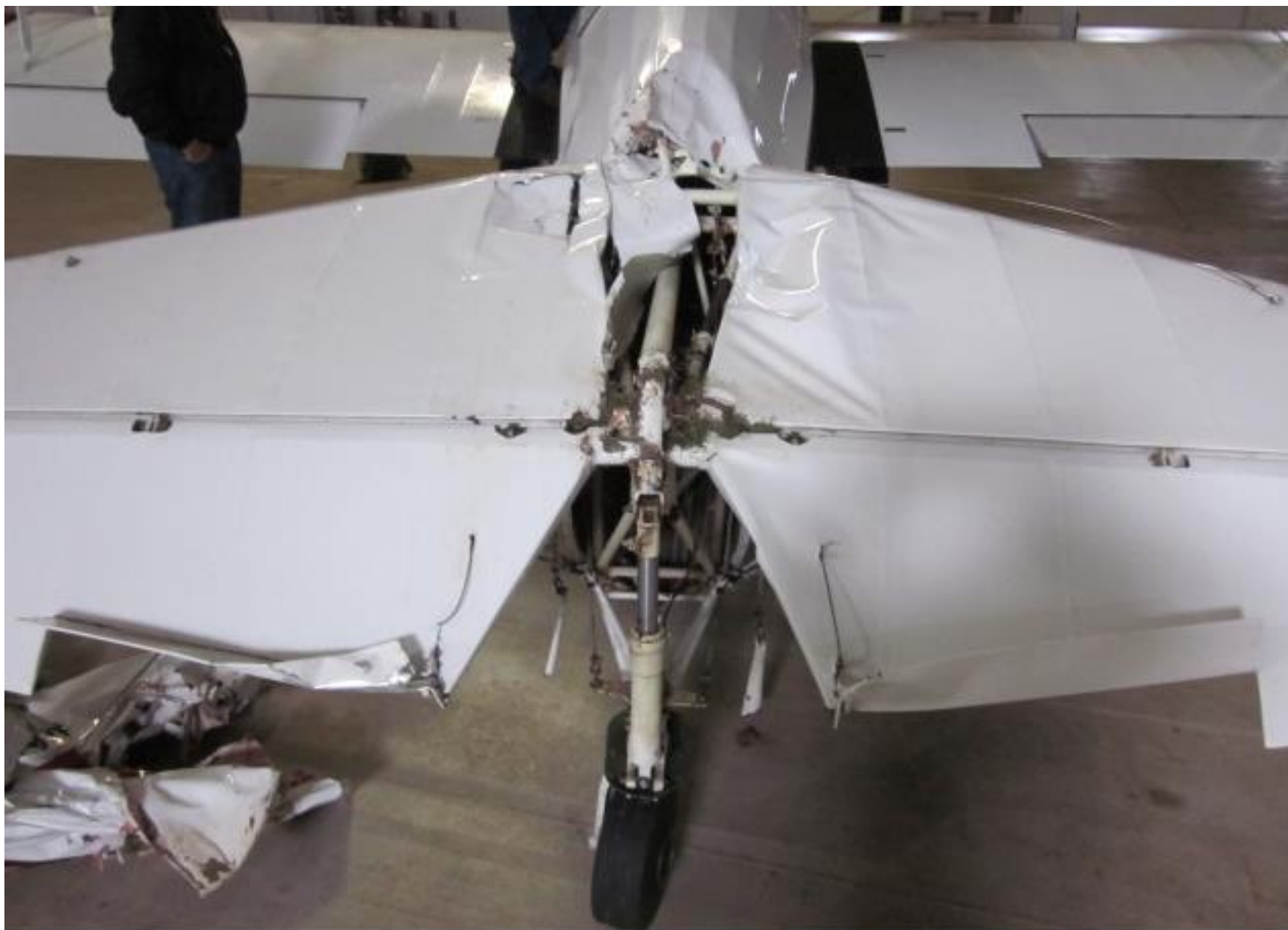
Photo 1 – View of damage to empennage and airframe (Photo courtesy of the FAA)
