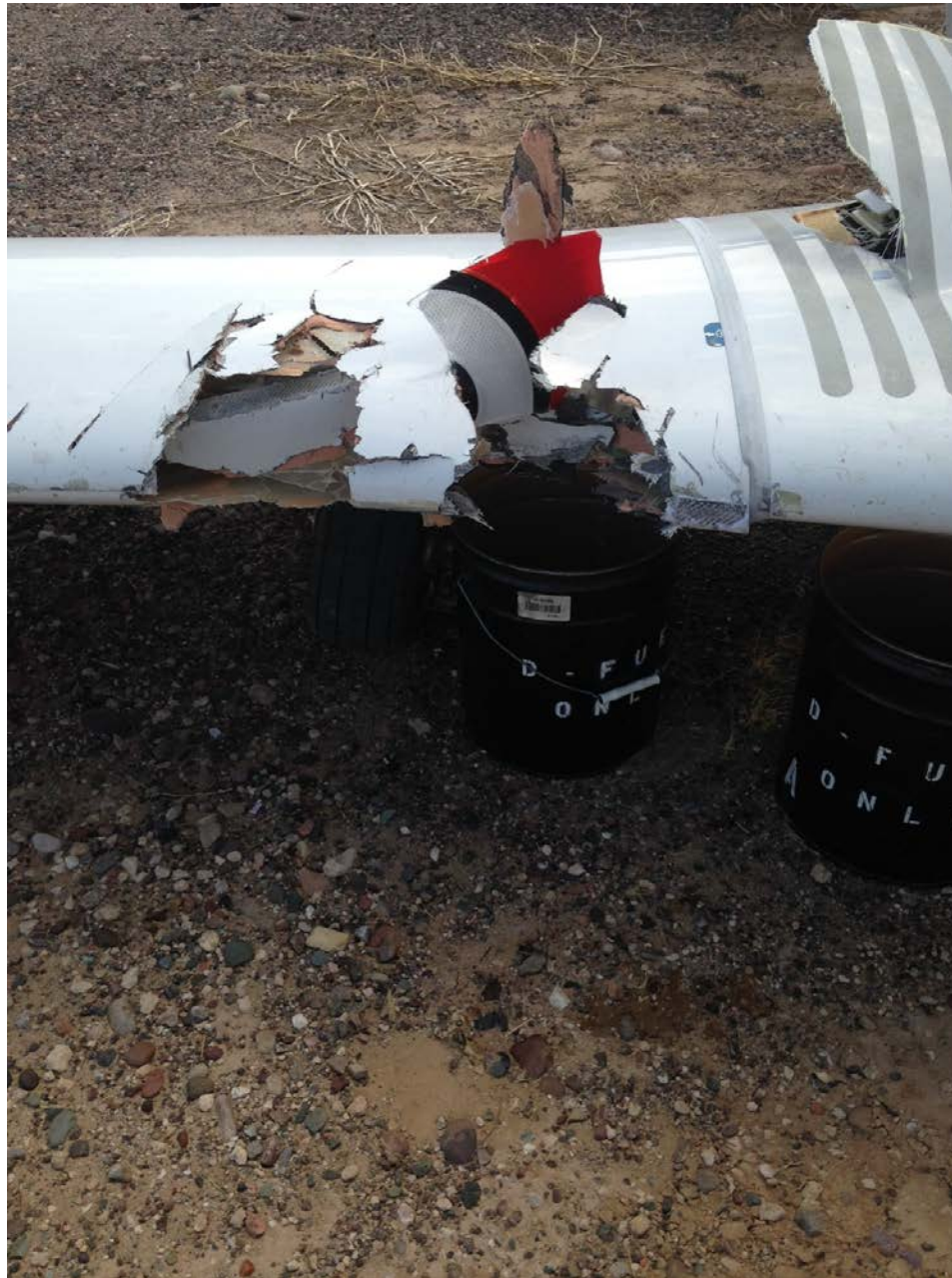
Photo 2 – View of damaged right wing leading edge with taxiway sign (photo courtesy unknown)
