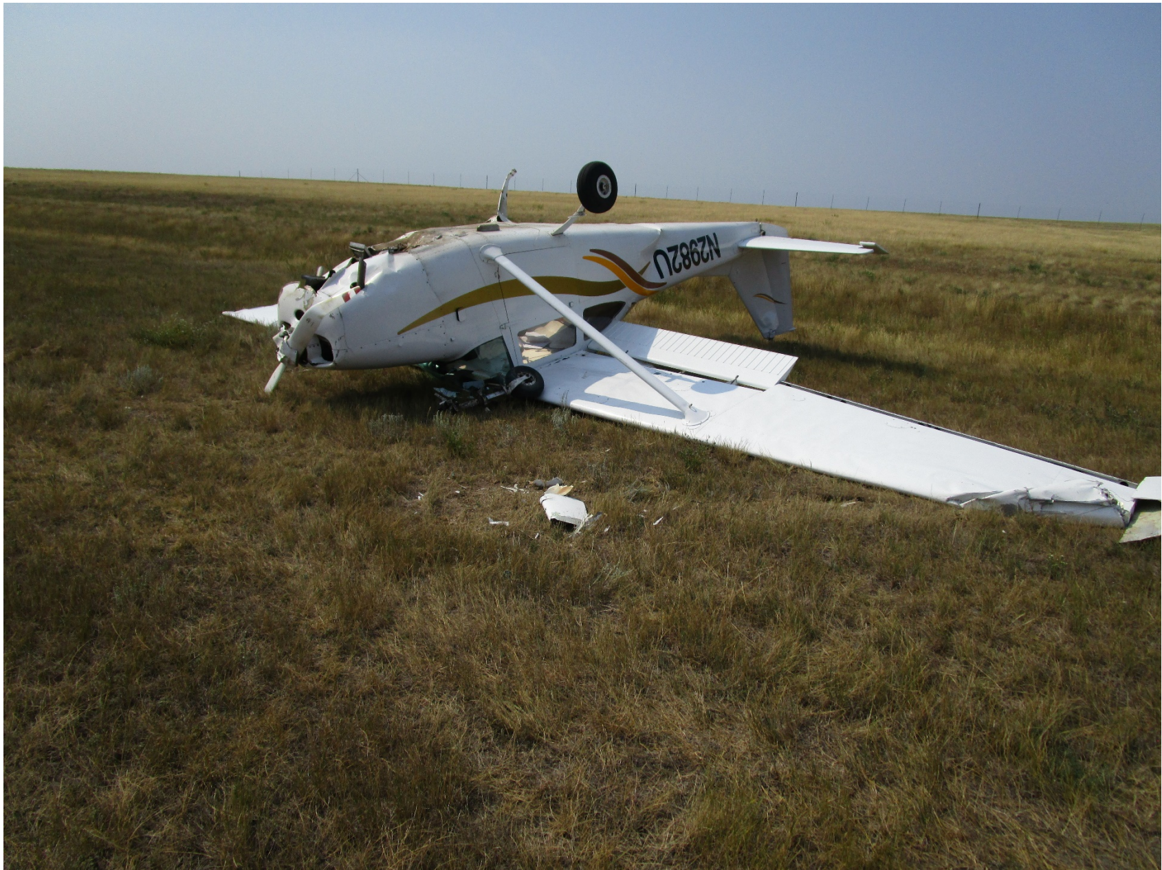
Photo 1 – Substantially Damaged Fuselage, Right Wing, and Vertical Stabilizer (Photo Courtesy of FAA)
