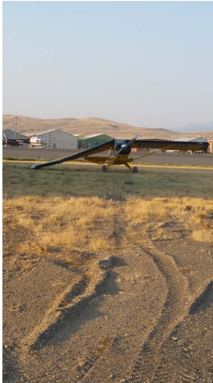
Photo 1 – View of damage to right wing struts and wing (Courtesy of FAA)
