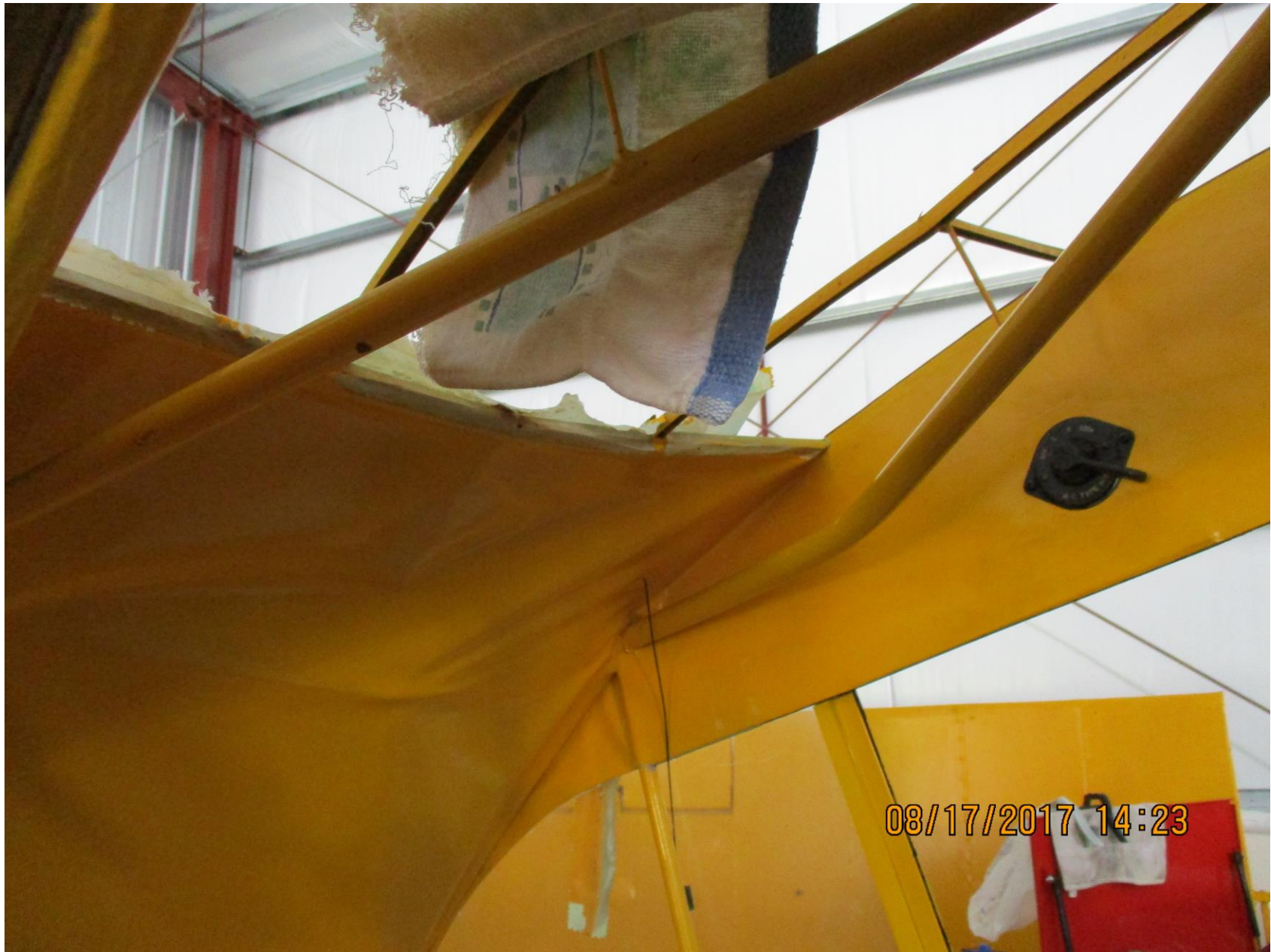
Photo 1 – Interior view of damaged airplane fuselage (Photo courtesy of the FAA)
