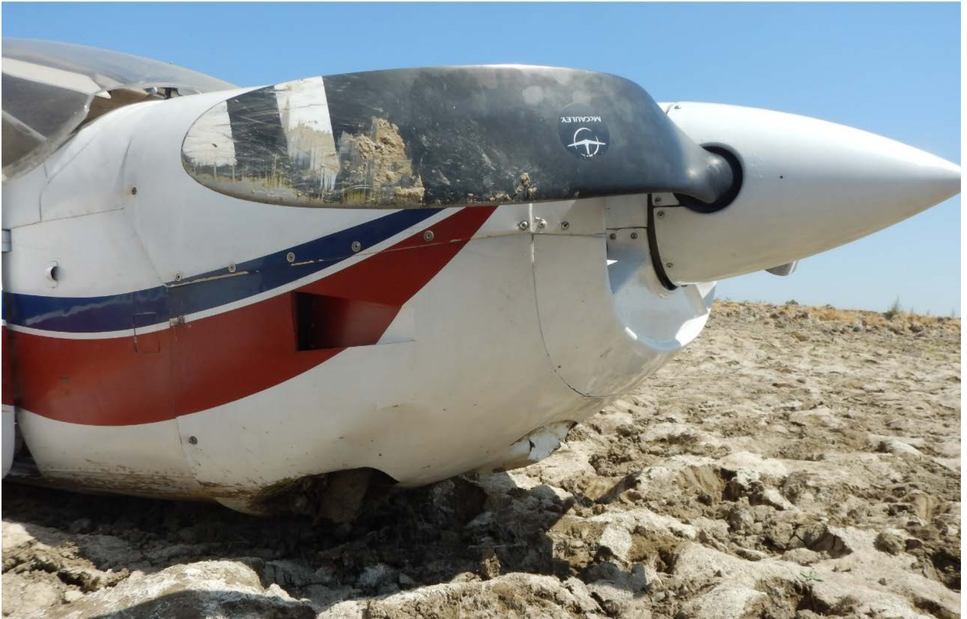
Photo 1 – View of damage to the windscreen (Courtesy of FAA)
