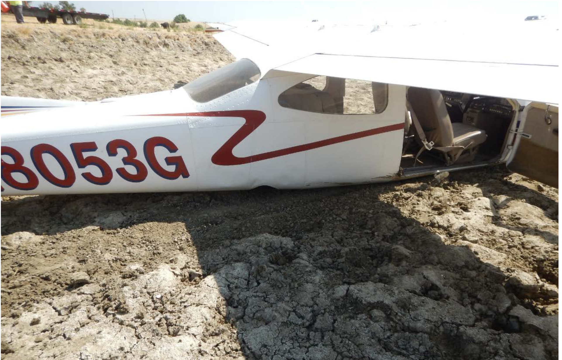
Photo 2 – View of damage to intermediate fuselage (Courtesy of FAA)
