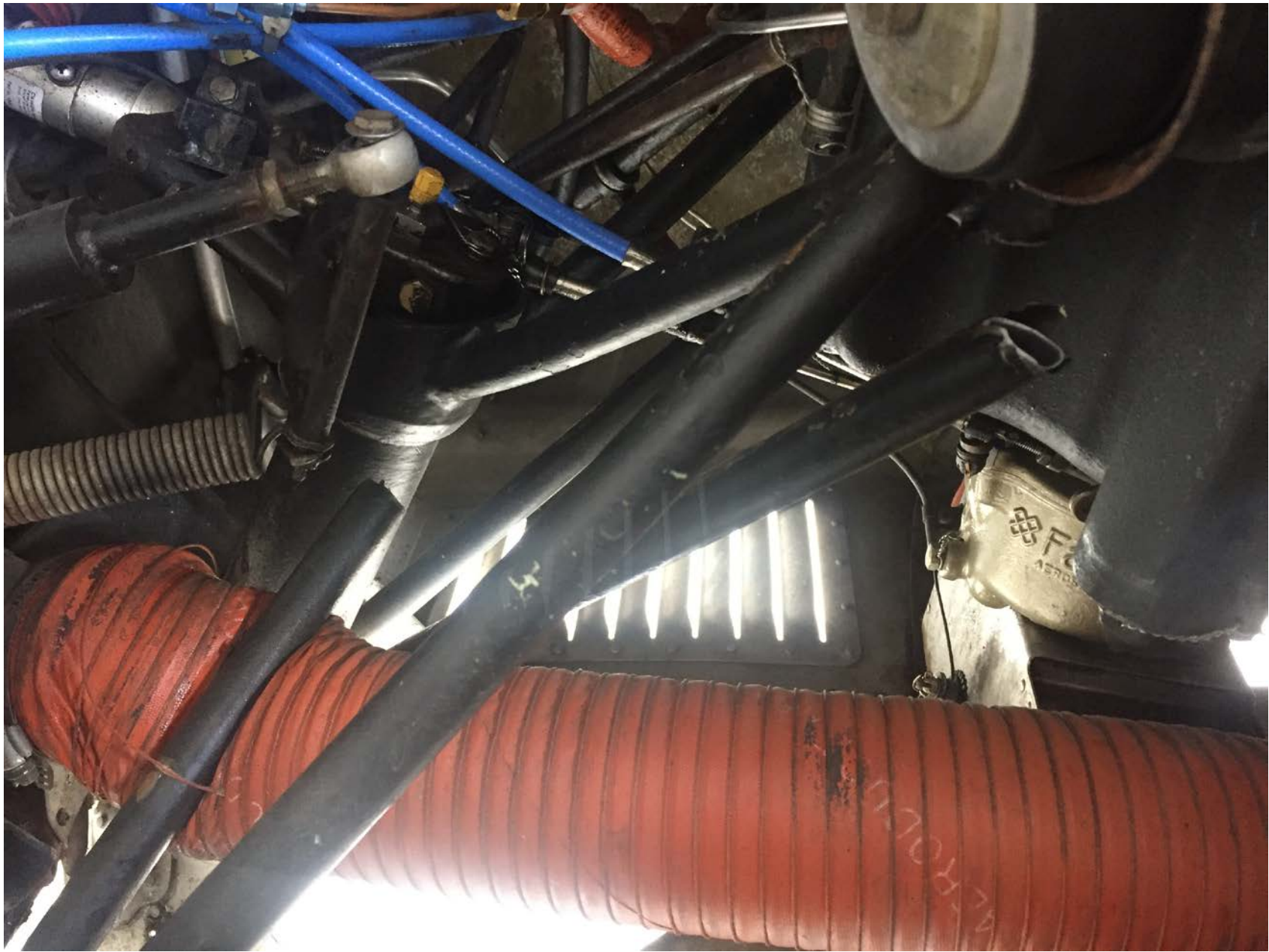
Photo 1 – View of damage to engine mounts (Courtesy of Operator)
