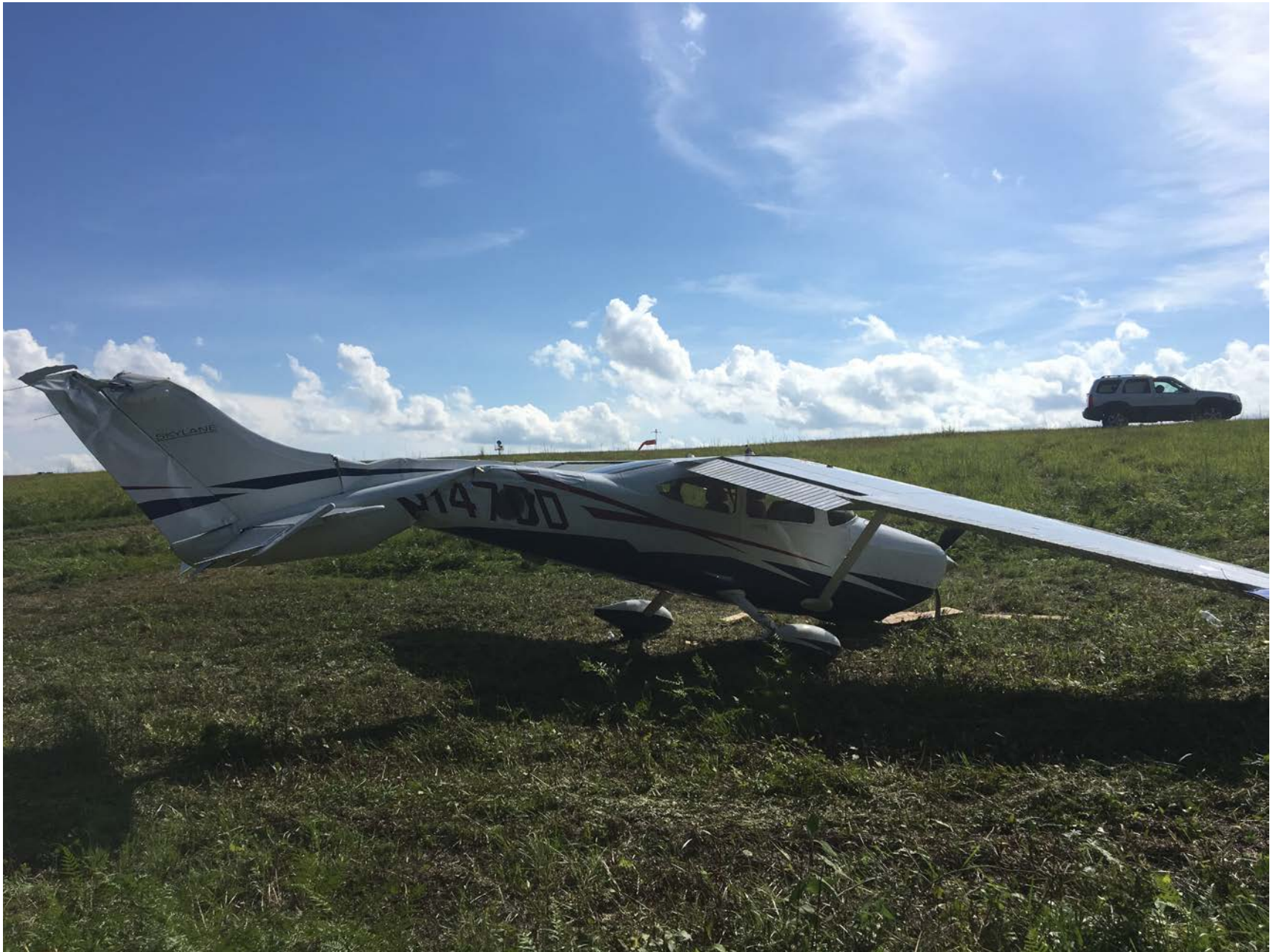
Photo 2 – View of damaged empennage and wings (photo courtesy of the FAA)
