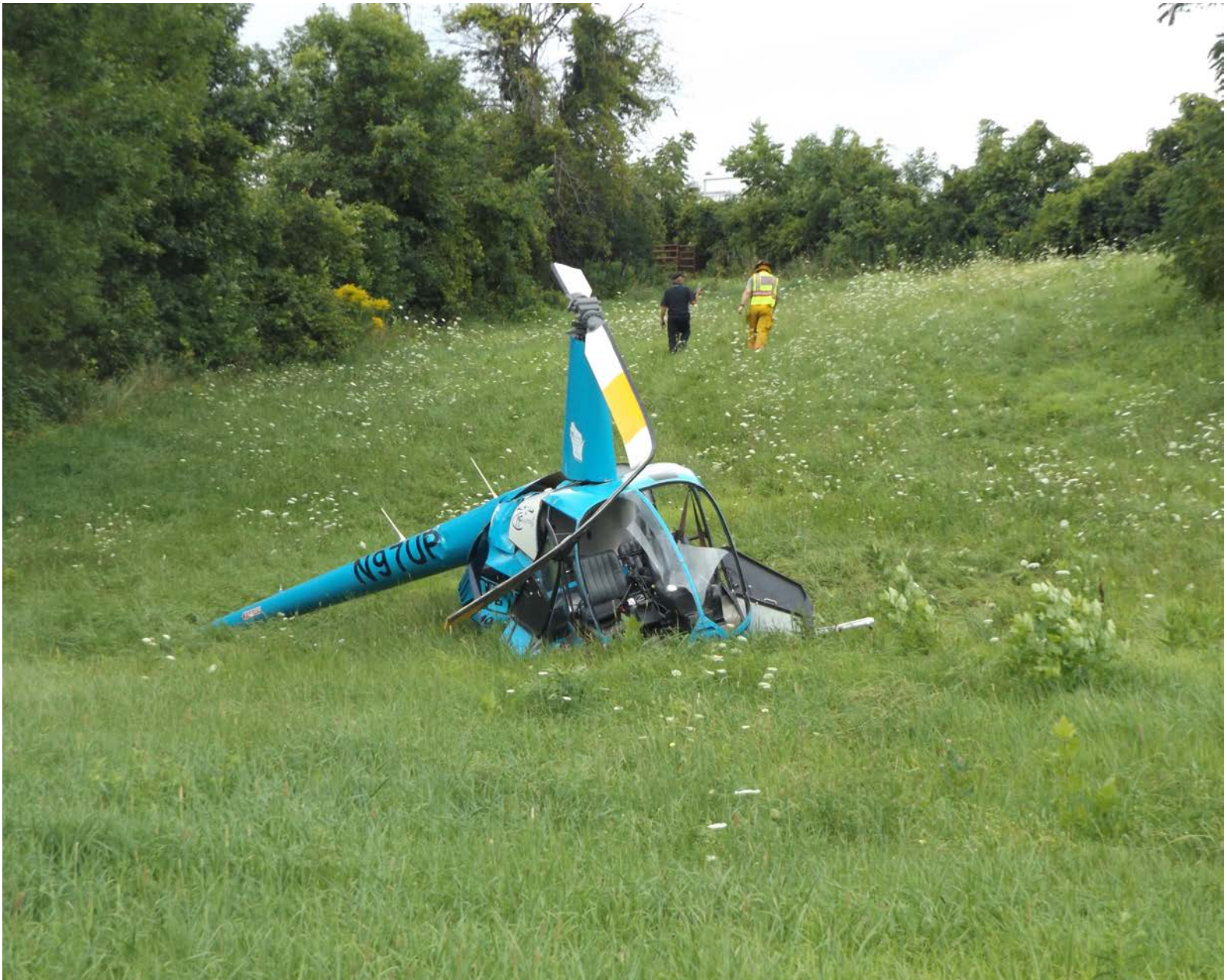
Photo 1 – Substantially Damaged Fuselage, Tail Boom, and Main Rotor (Photo Courtesy of FAA)
