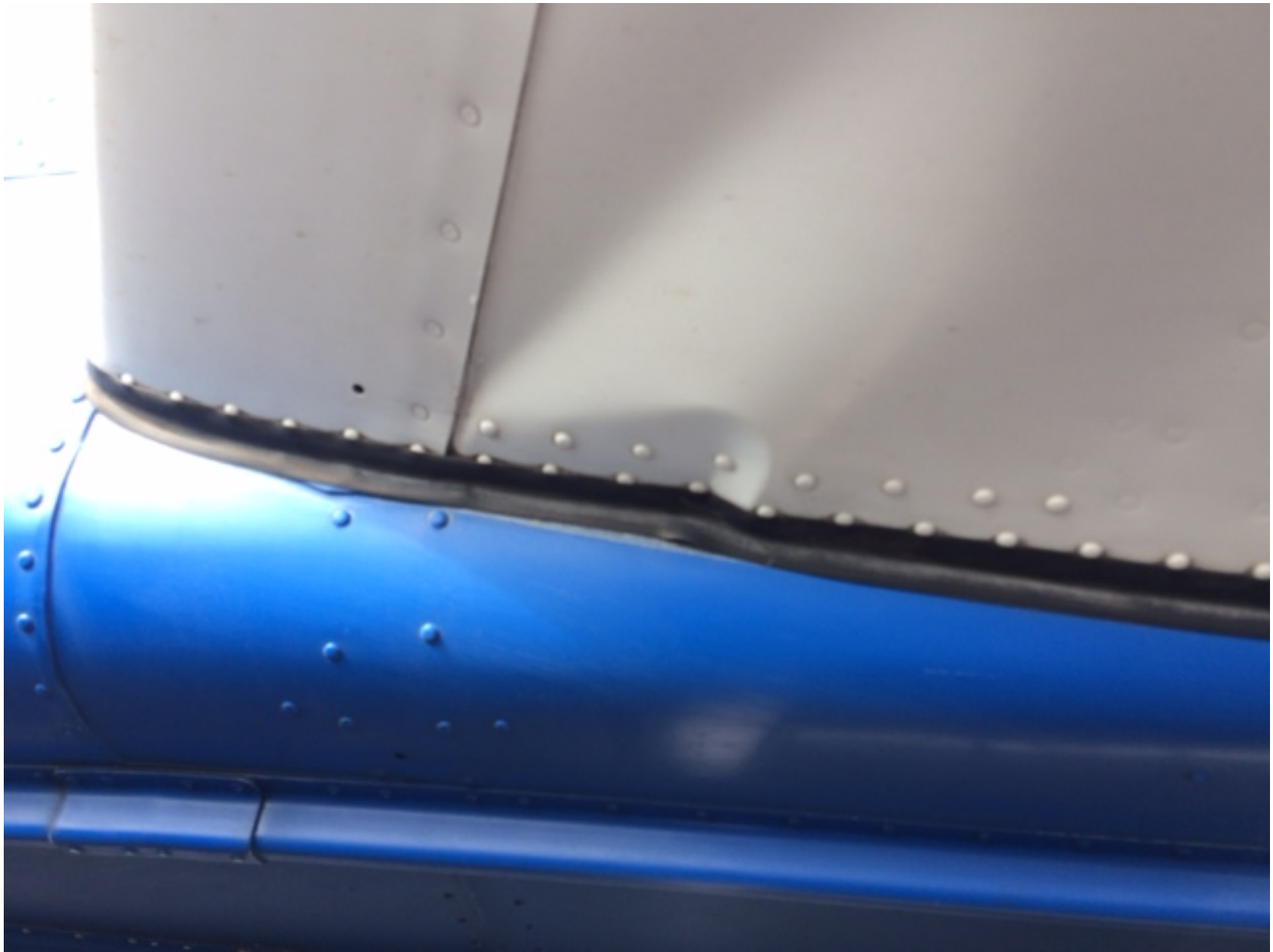
Photo 2 - Underside of the Substantially Damaged Left Wing (Photo Courtesy of FAA)
