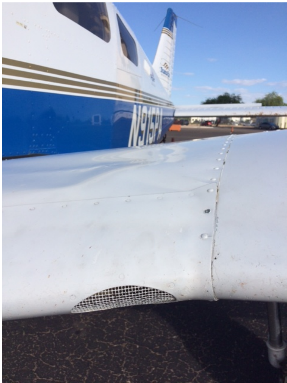
Photo 1 – Substantially Damaged Left Wing (Photo Courtesy of FAA)
