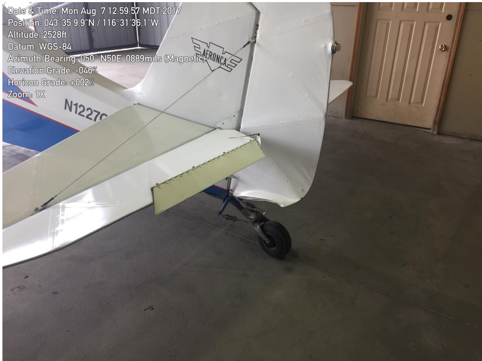
Photo 1 – View of rudder damage (photo courtesy of the FAA).
