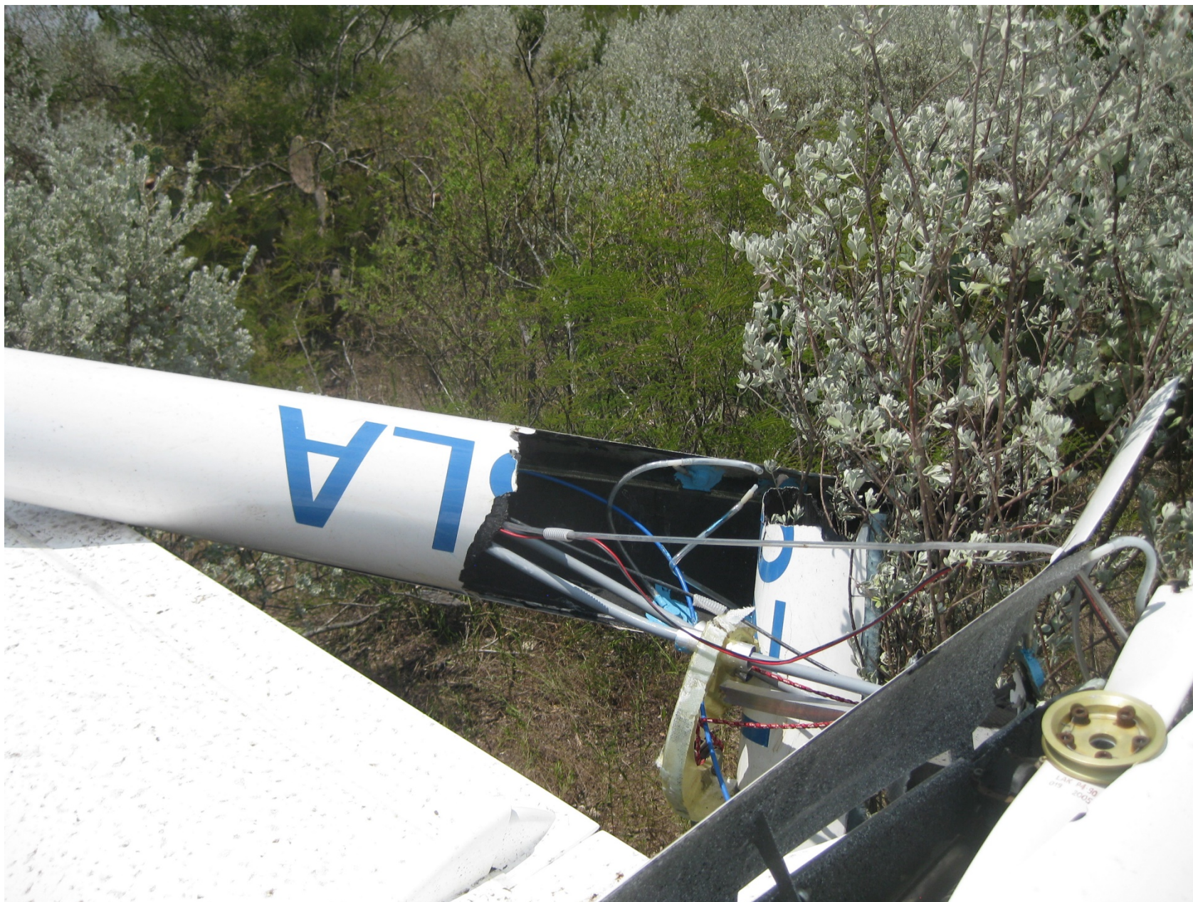
Photo 1 – Substantially Damaged Fuselage (Photo Courtesy of FAA)
