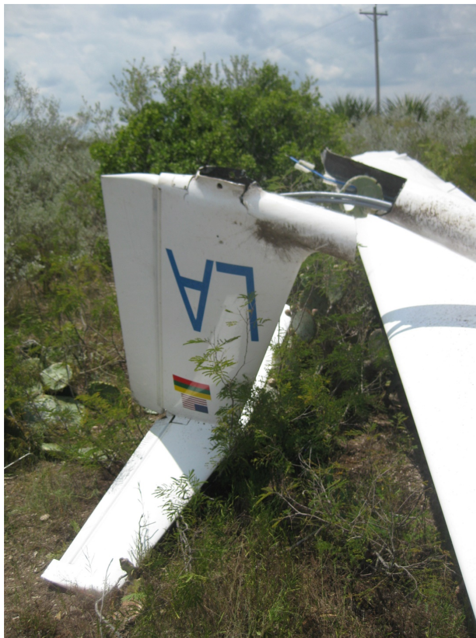
Photo 2 - Substantially Damaged Empennage (Photo Courtesy of FAA)
