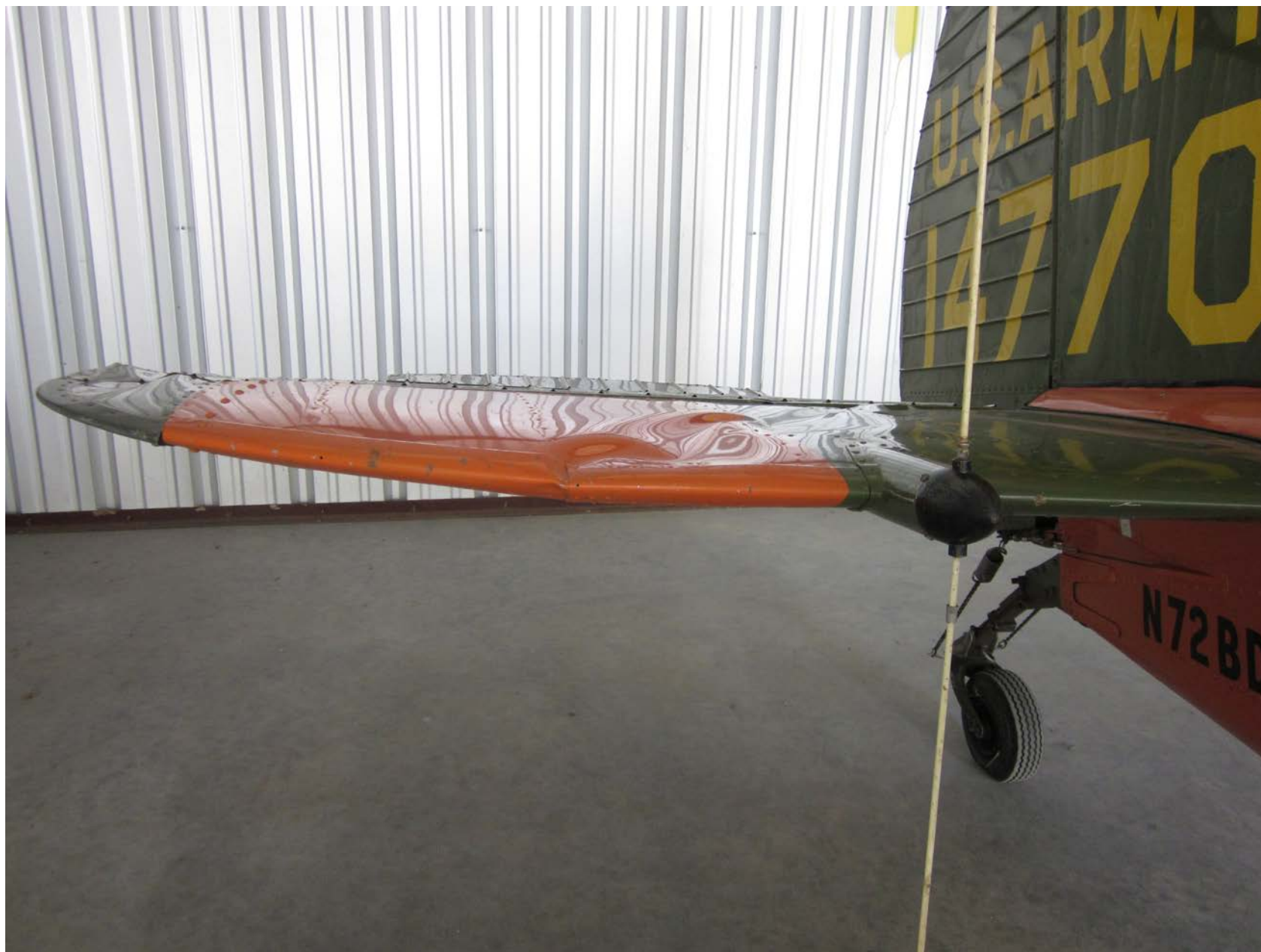
Photo 1 – View of damage to horizontal stabilizer (Courtesy of FAA)
