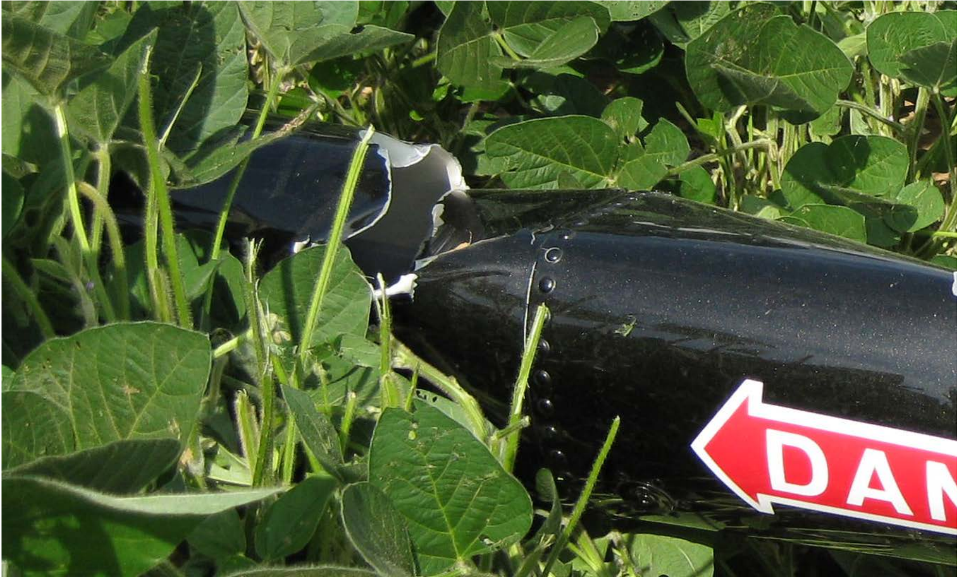
Photo 1 – View of damage to tailboom (Courtesy of FAA)
