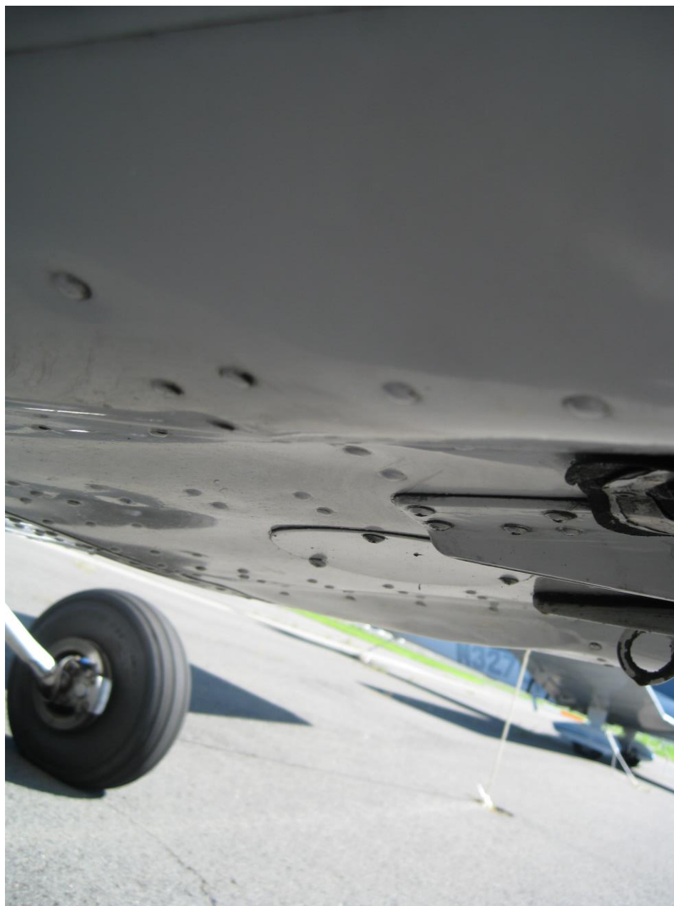
Photo 1 – View of fuselage damage (photo courtesy of the FAA)
