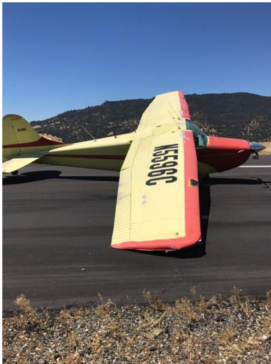
Photo 2 – View of straight tailwheel (Photo courtesy of the FAA)
