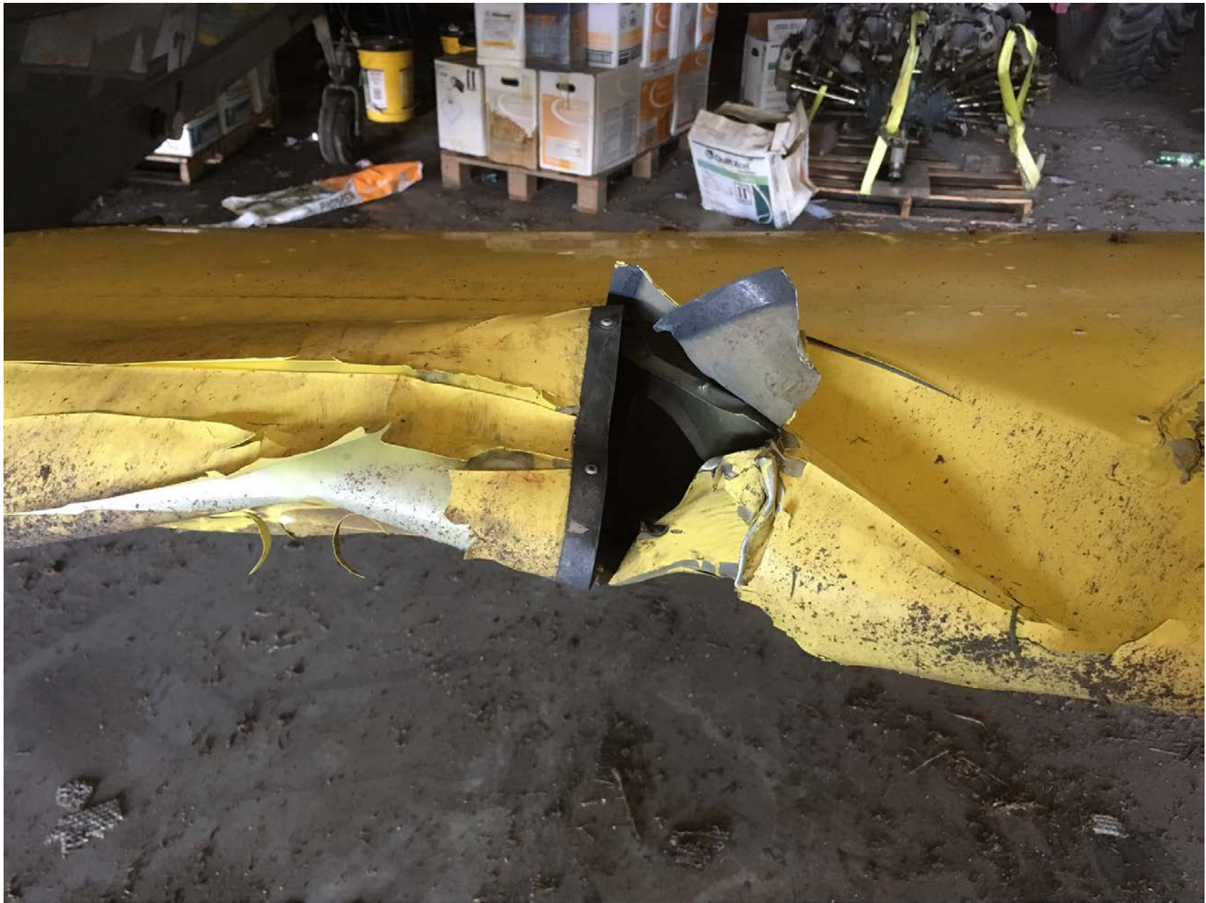
Photo 2 – View of damaged inboard lower left wing (photo courtesy of the FAA)
