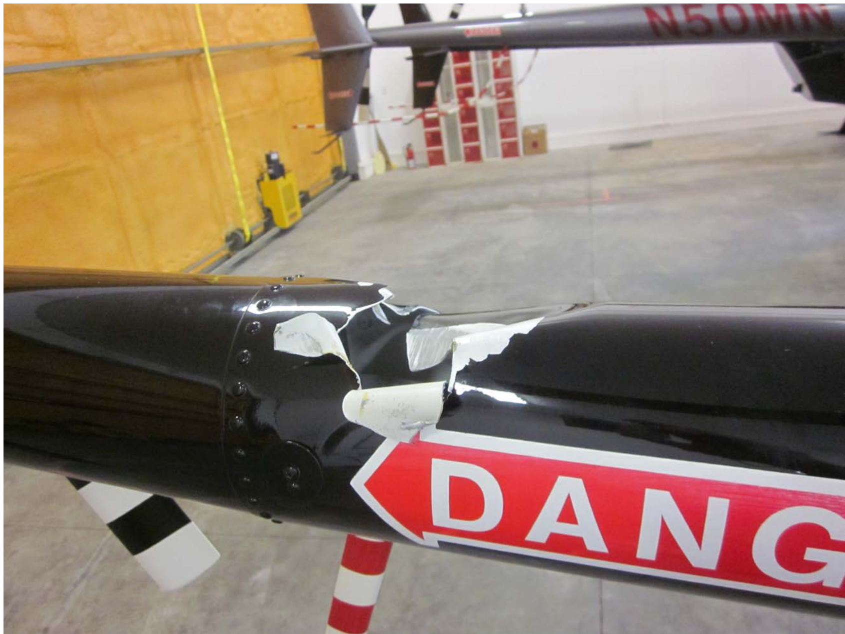
Photo 1 – View of damage to tailboom (Courtesy of FAA)
