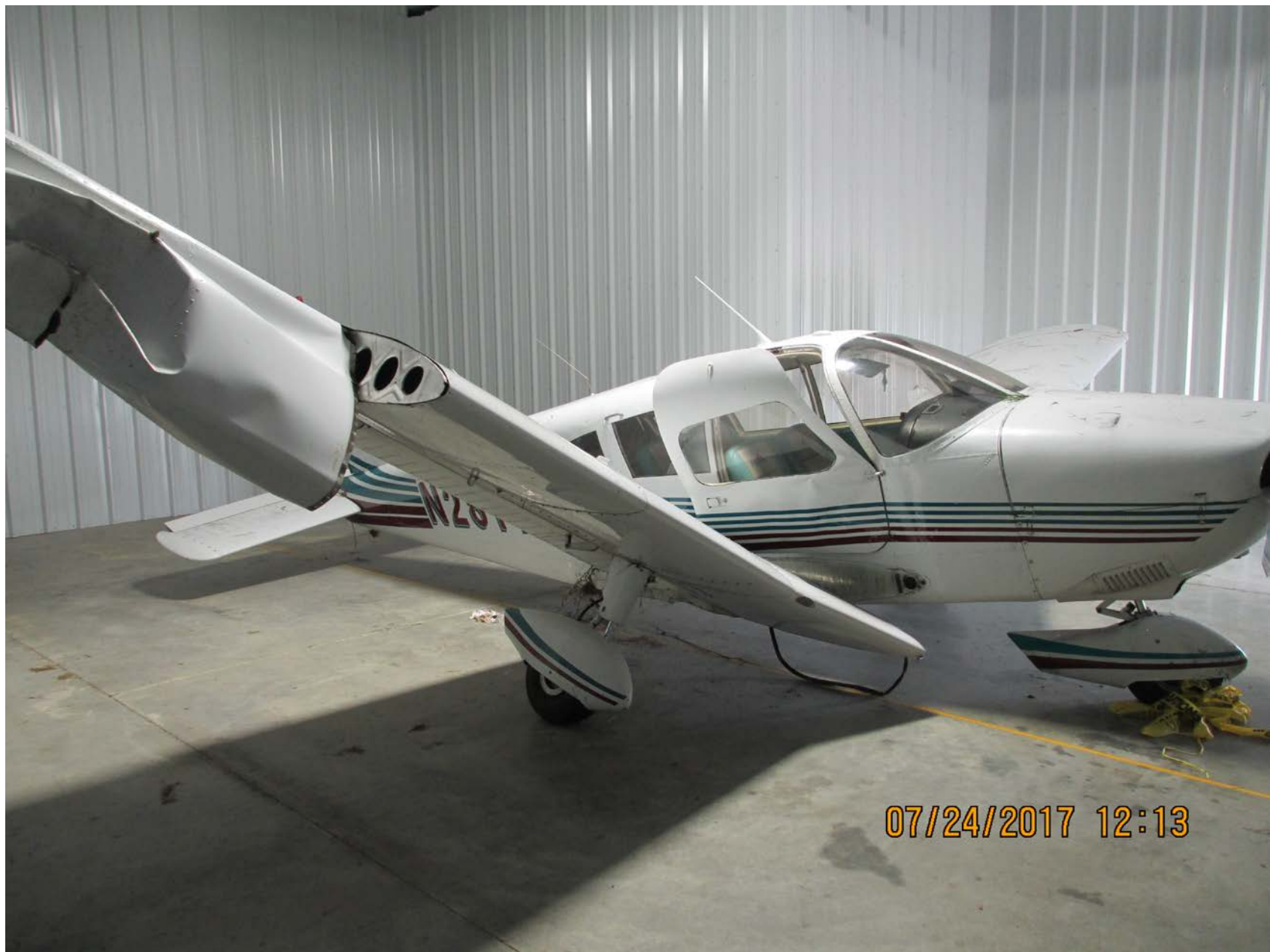
Photo 1 – View of damage to right wing spar and leading edge (Courtesy of FAA)
