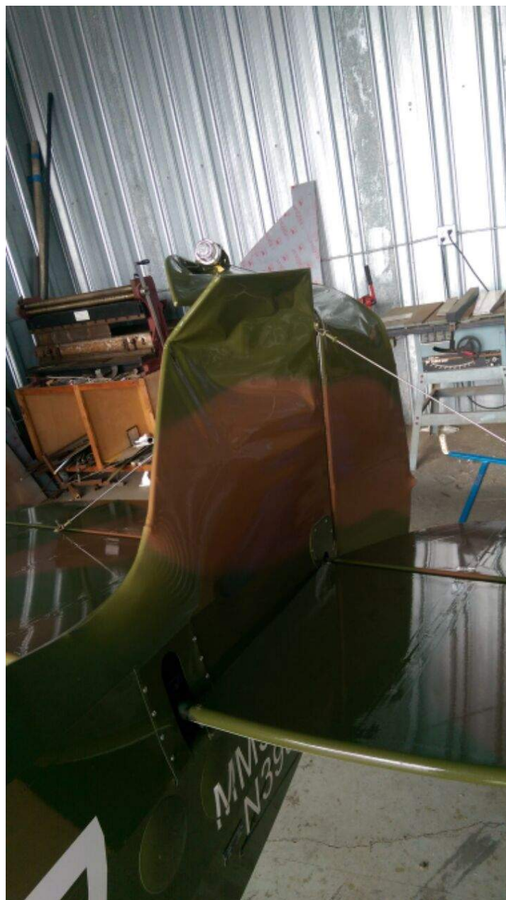
Photo 1 – View of damage to vertical stabilizer and rudder (Courtesy of FAA)
