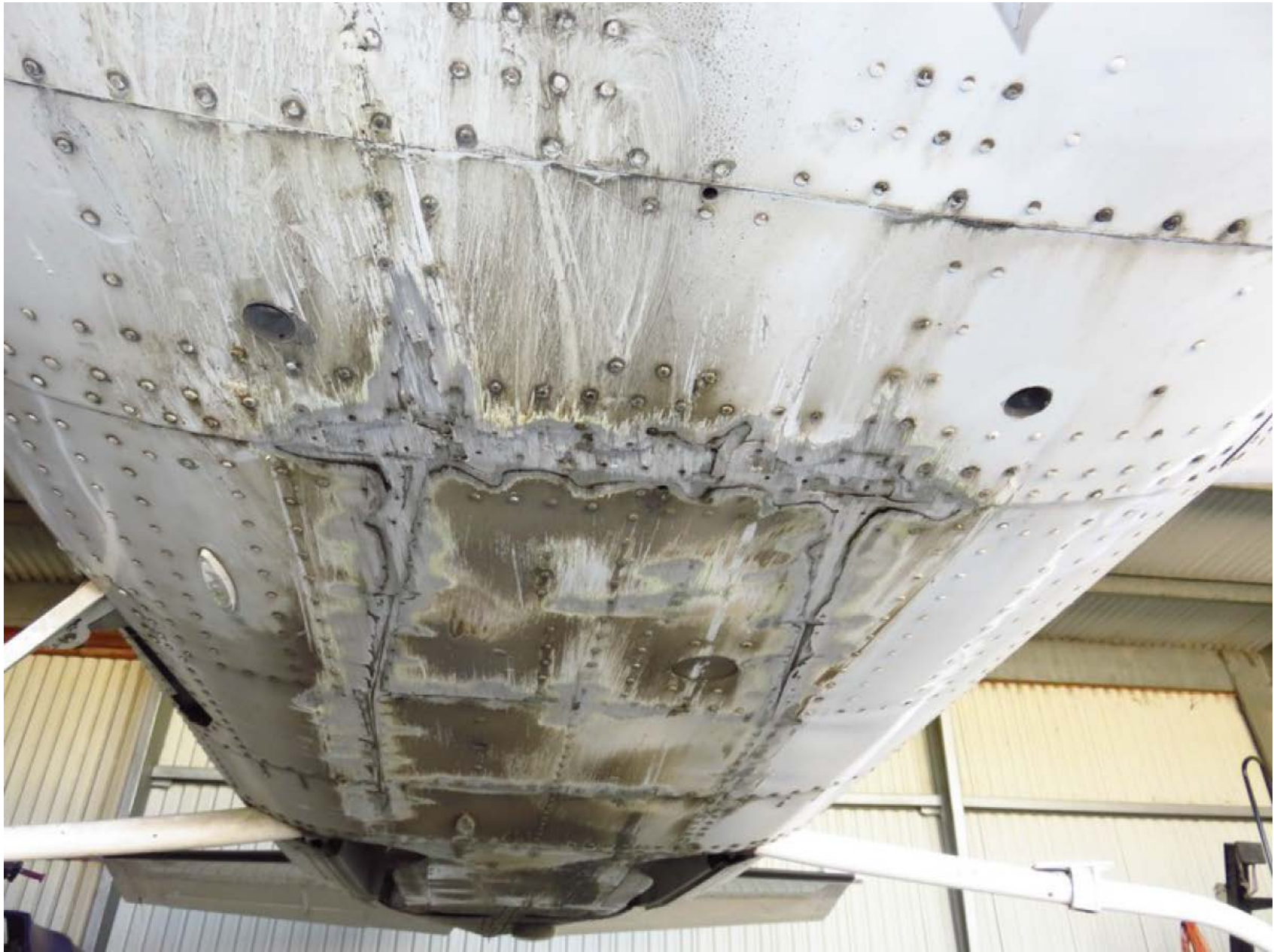
Photo 1 – View of damage to longerons and formers (Courtesy of FAA)
