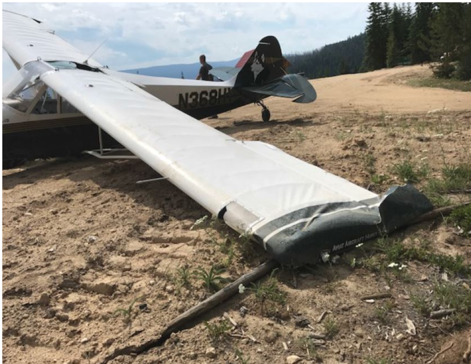
Photo 2 - Substantially Damaged Left Aileron and Left Elevator (Photo Courtesy of FAA)
