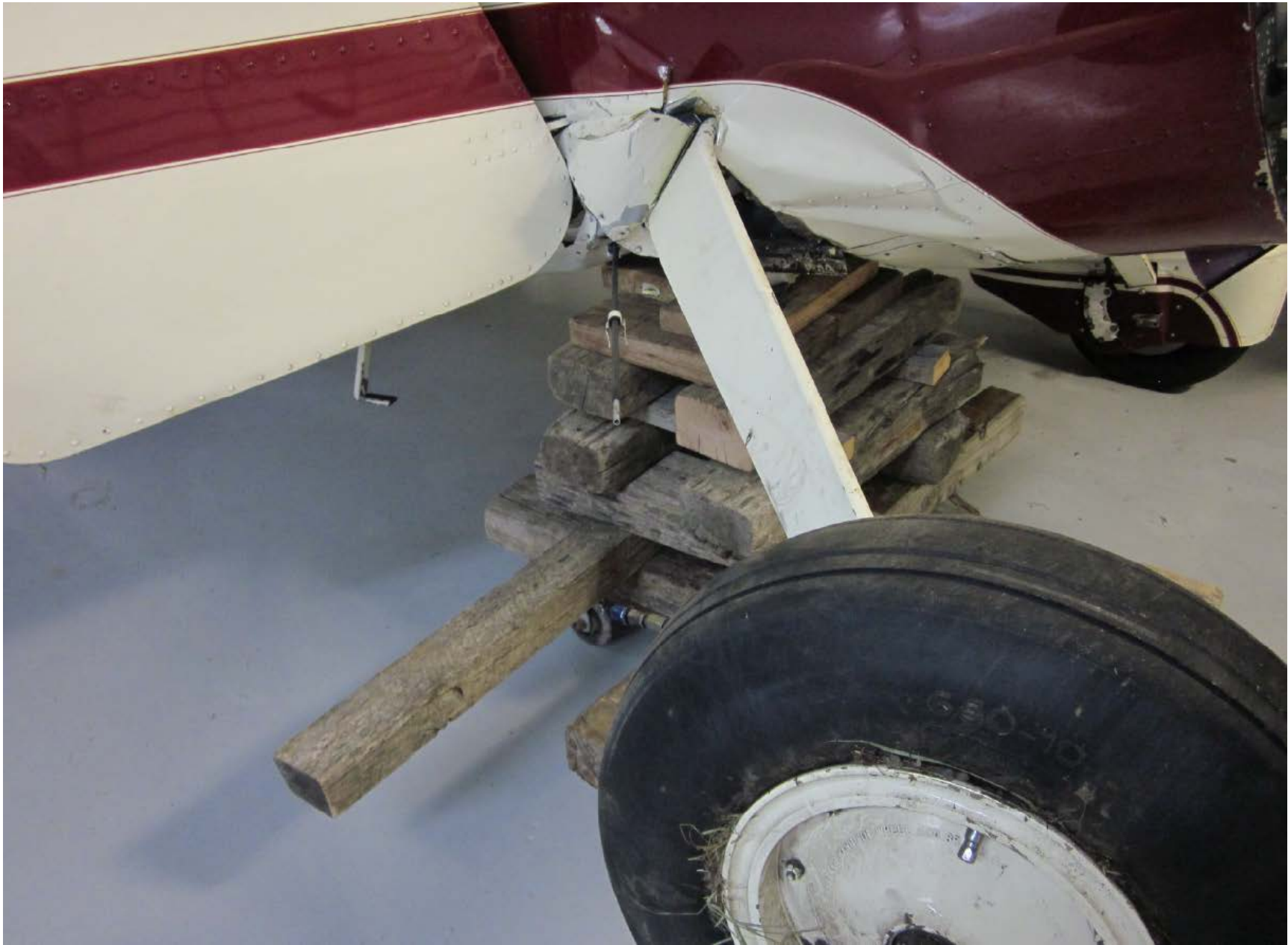
Photo 1 – View of damage to the right main landing gear attachment points (Courtesy of FAA)
