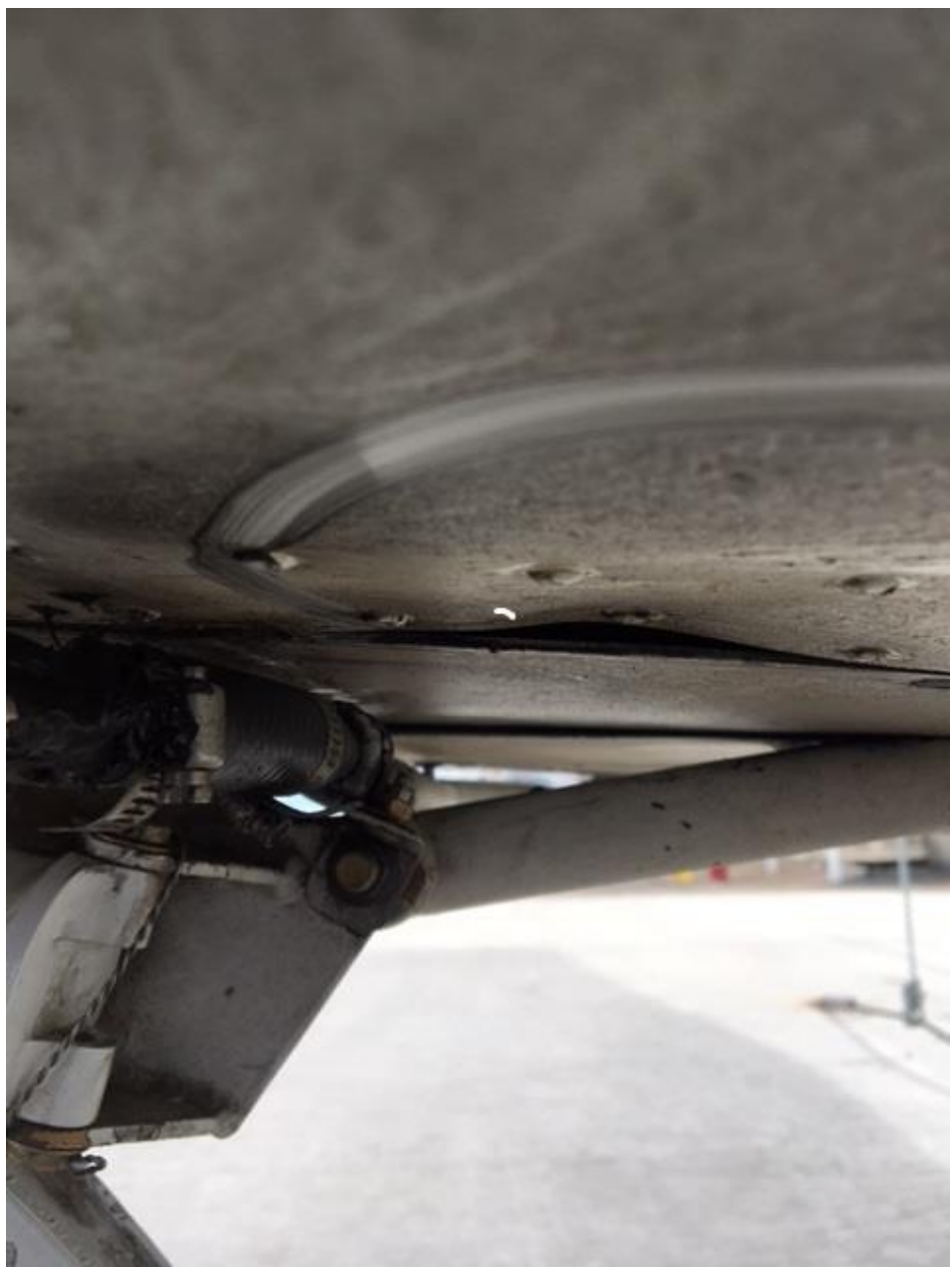
Photo 1 – View of damage by front landing gear (Photo courtesy of Forest Service)
