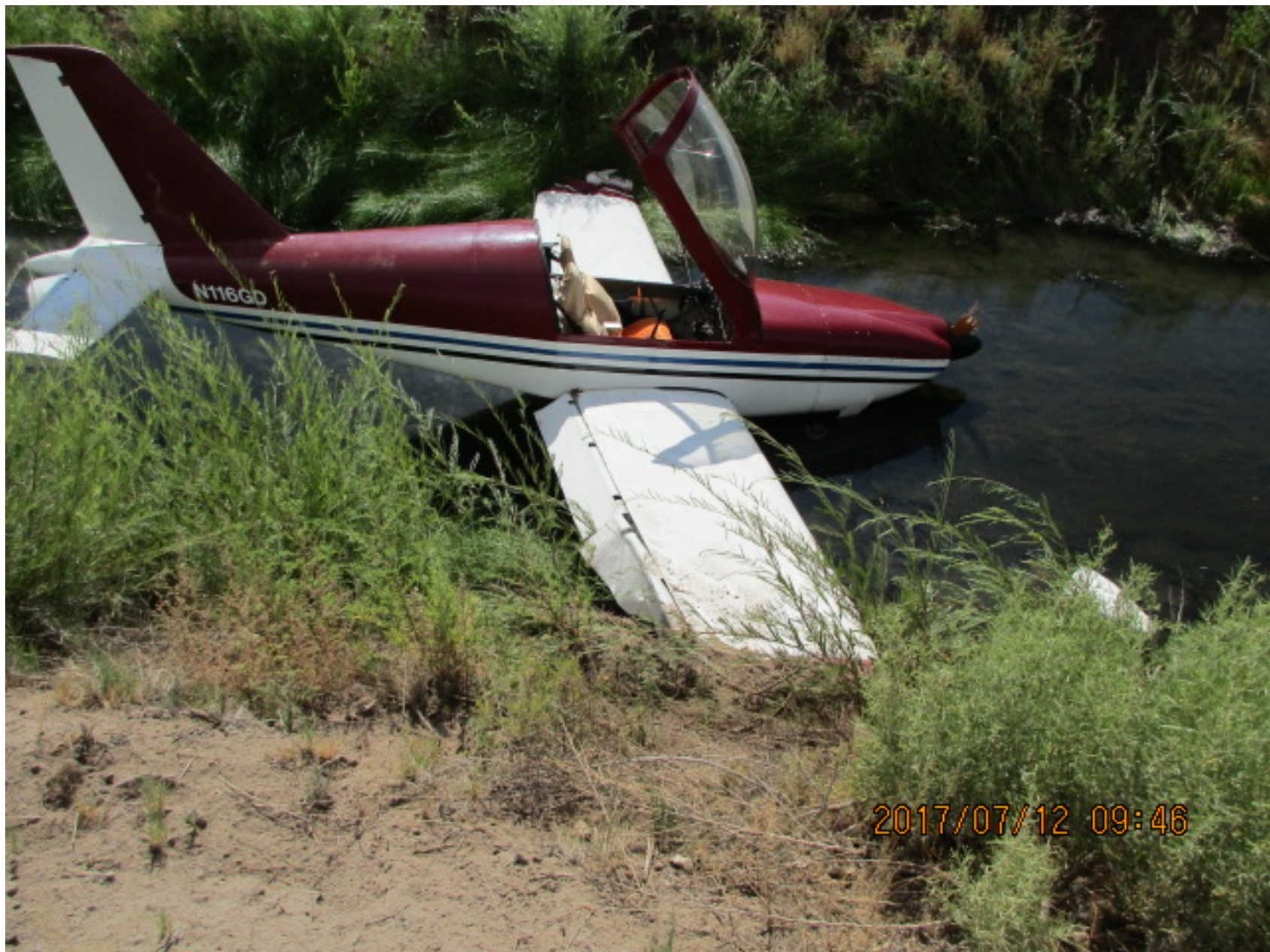
Photo 1 – Substantially Damaged Wings, Aileron, and Elevator (Photo Courtesy of FAA)
