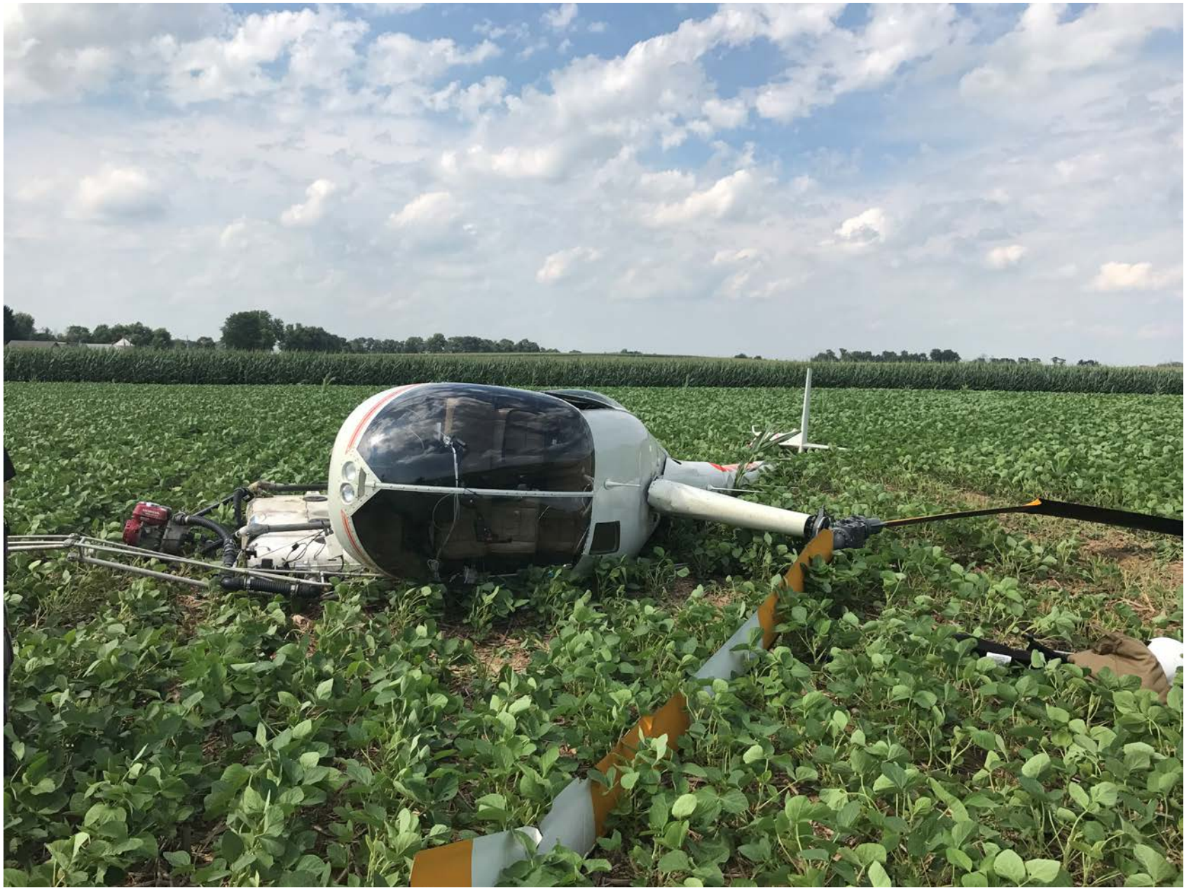
Photo 1 – View of damage to the main rotor system and the tailboom (Courtesy of Operator)
