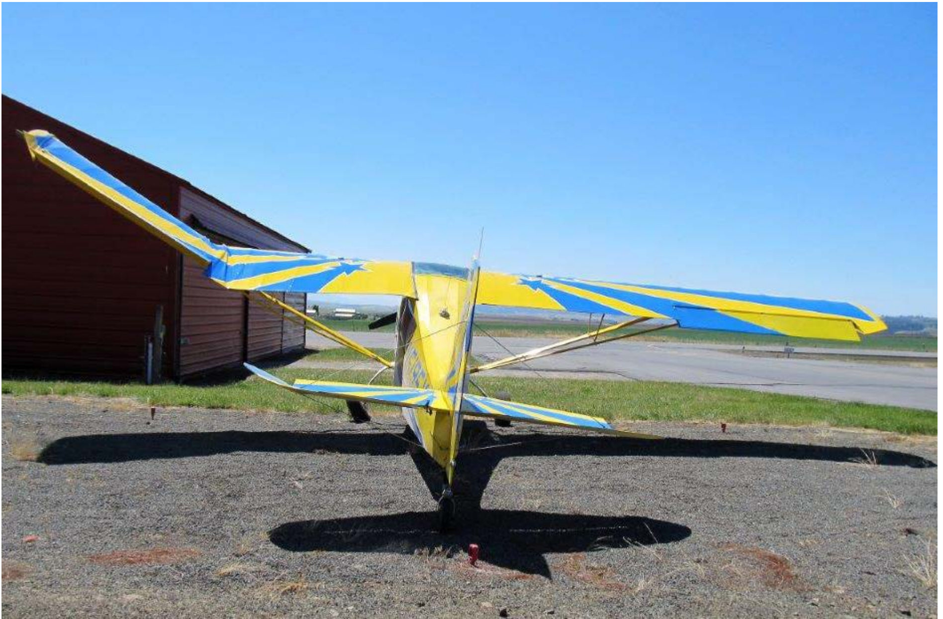
Photo 1 – View from rear of left wing and elevator damage (photo courtesy unknown)
