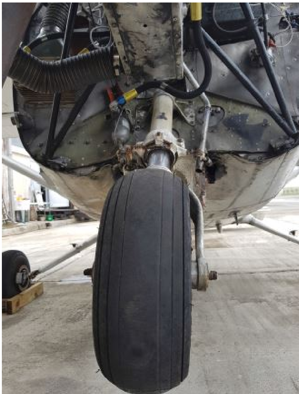
Photo 1 – Substantially Damaged Firewall (Photo Courtesy of FAA)
