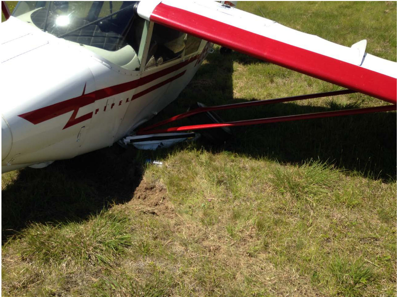
Photo 1 – View of damaged left wing lift struts (photo courtesy of the FAA)
