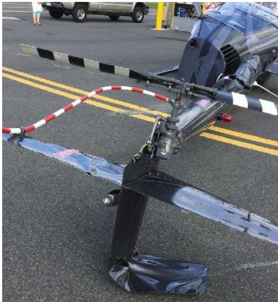
Photo 1 – View of damage to the vertical and horizontal stabilizer and the tail rotor drive shaft (Courtesy of FAA)
