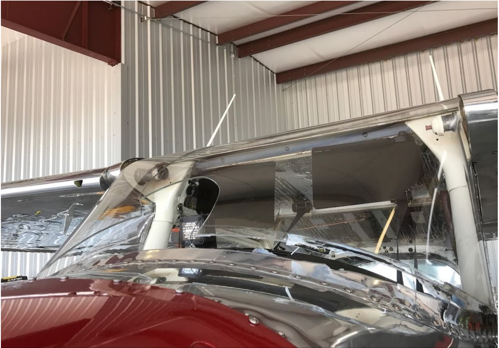
Photo 2 - Substantially Damaged Windscreen (Photo Courtesy of FAA)
