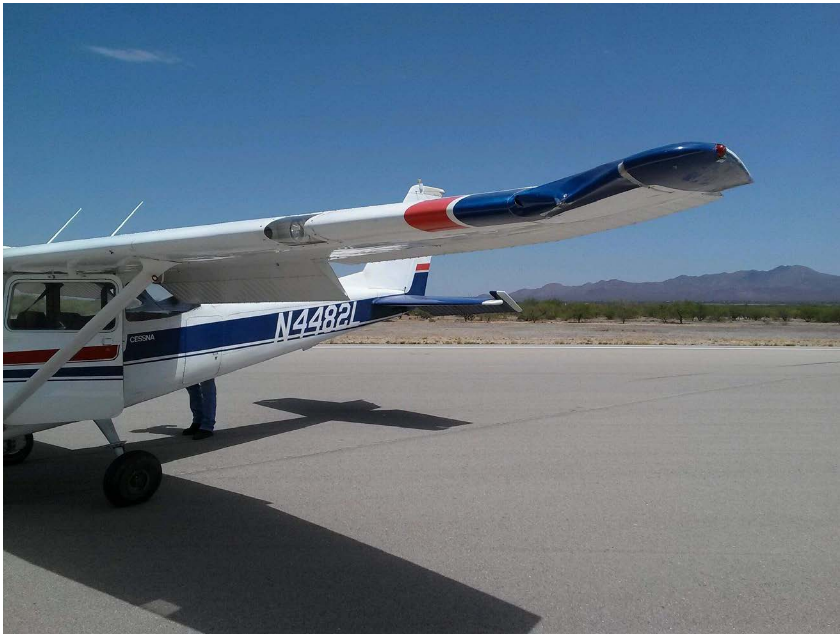
Photo 1 – View of damaged left wing (photo courtesy unknown)
