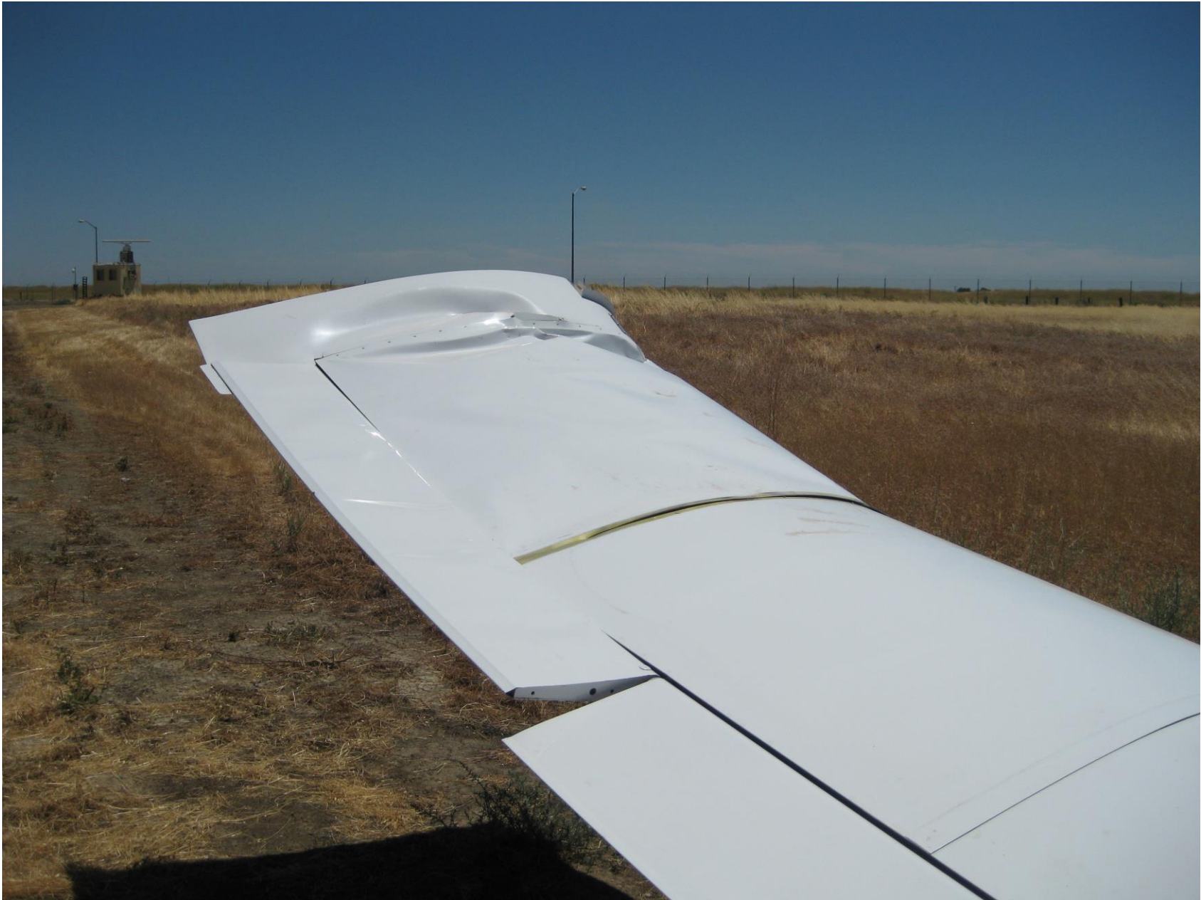
Photo 1 – Rear view of damaged left wing (Photo courtesy of the FAA)
