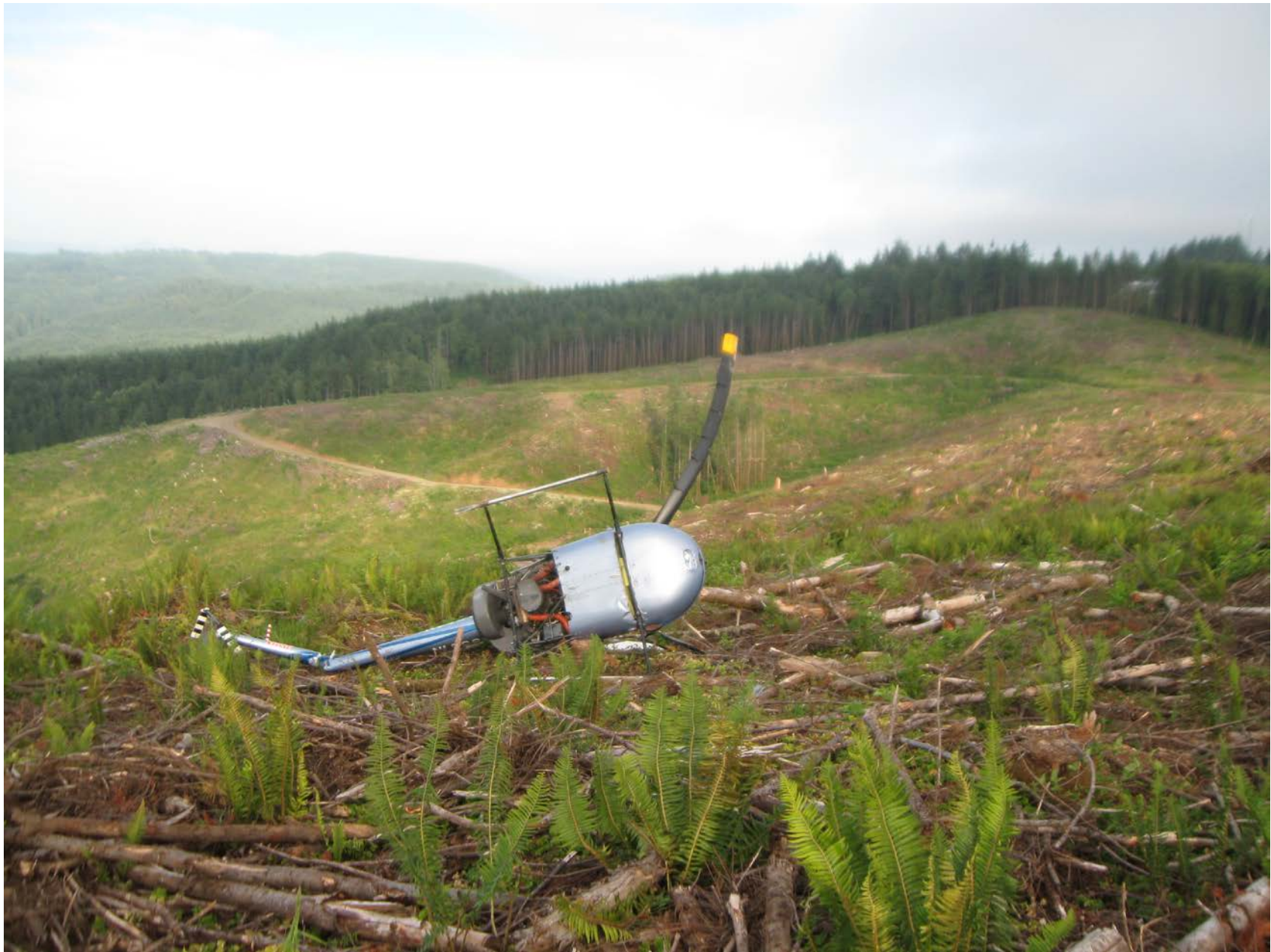
Photo 1 – View of damage to the tail rotor drive shaft and the main and tail rotor blades (Courtesy of FAA)
