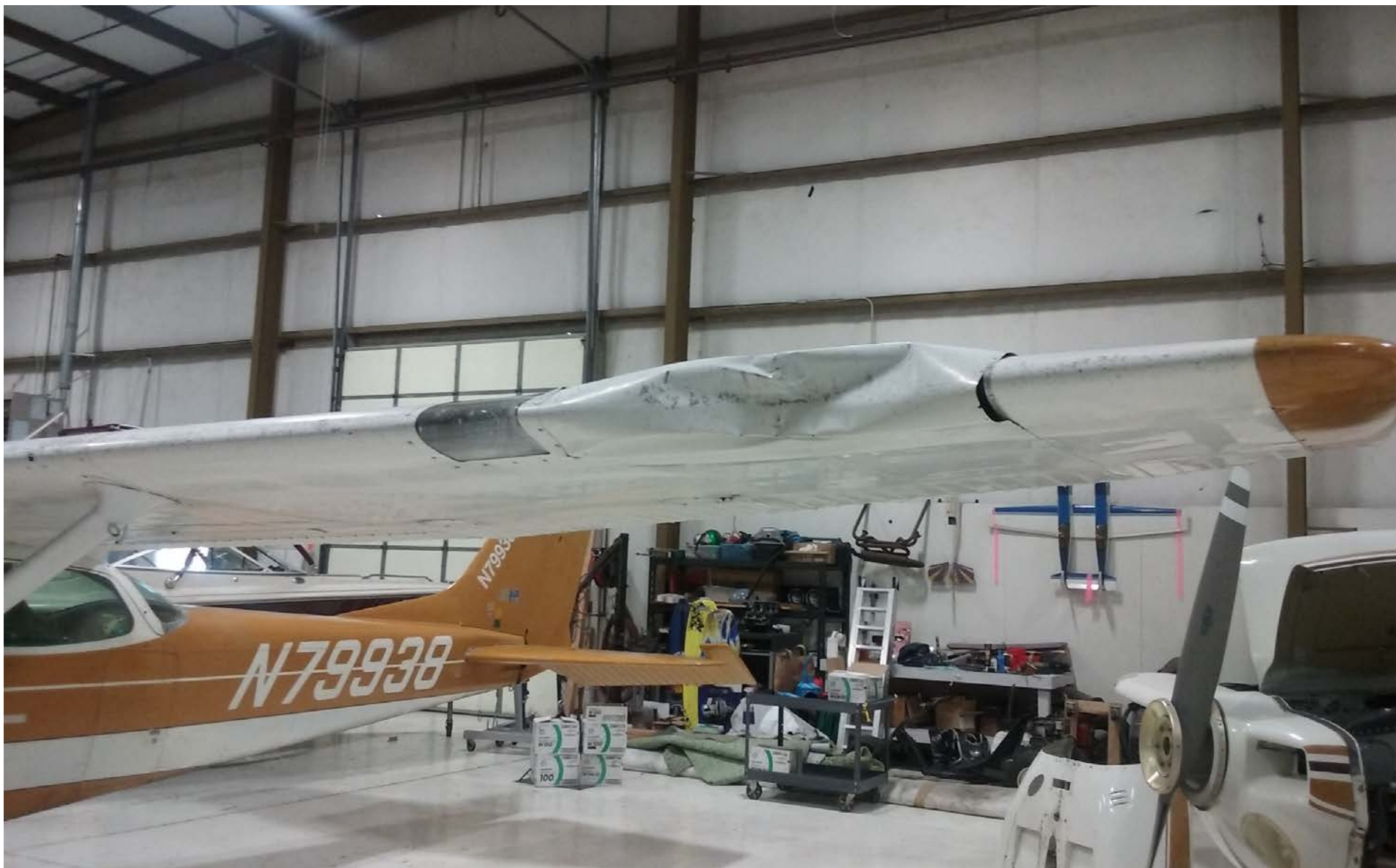
Photo 1 – View of damage to left wing rib and leading edge (Courtesy of FAA)
